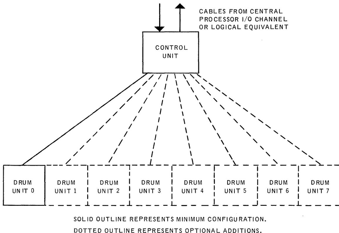
Figure 2-1. Block Diagram of FH-880 Drum Subsystem
