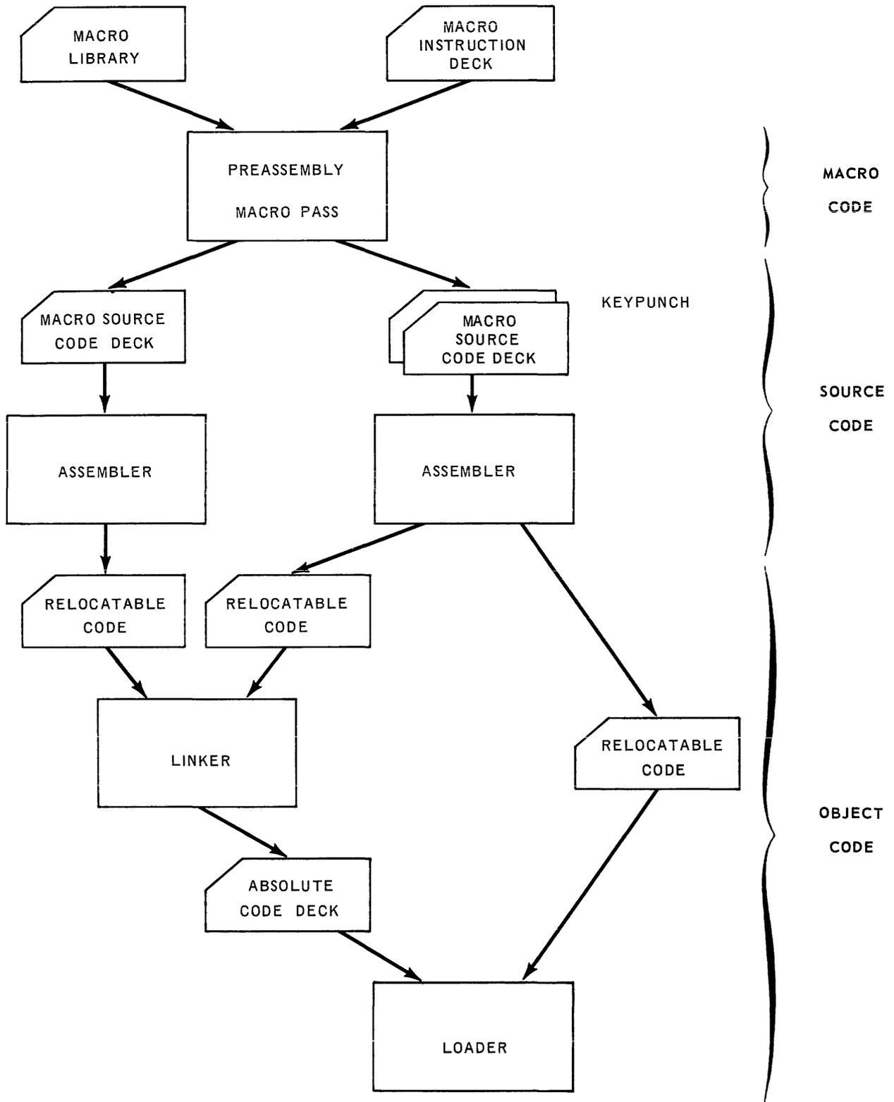
Figure 1-2. 9200/9300 Assembly System
