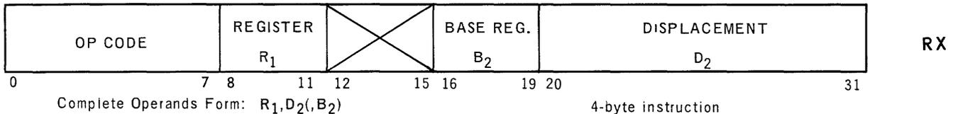
In general, instructions in this format are used to process data between registers and storage, and include such functions as load, store, compare, add, subtract and branch. The mnemonic codes for instructions using this type of format are:
