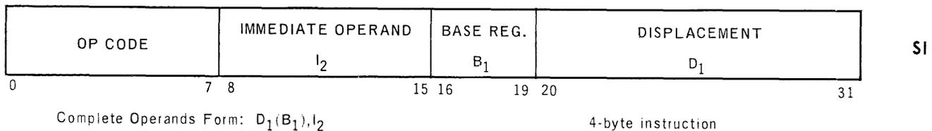
In general, instructions with this format are used for processing with control data contained in the instruction. The mnemonic codes for instructions using this type of format are:
