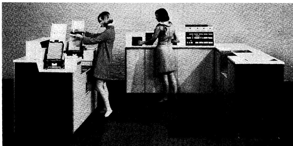
*This card-oriented UNIVAC 9300 system includes the dual-feed 1001 Card Controller (left) as well as the basic card reader and punch (at right). The 600-lpm printer is an integral part of the processor cabinet (center). A variety of disc drives, magnetic tape units, and other peripheral equipment can be added.*
