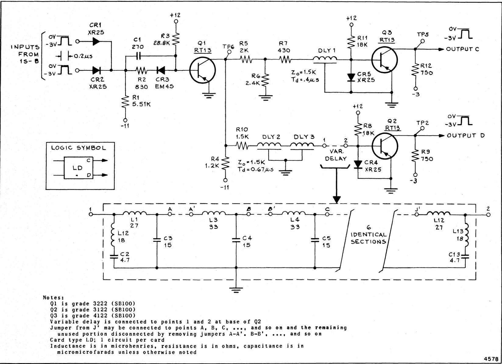
Figure 1-34. Long-Delay Circuit
