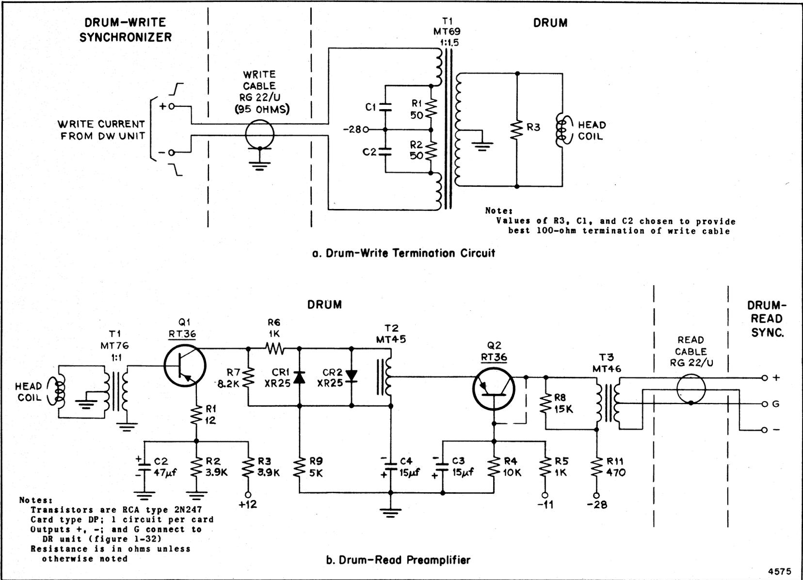
Figure 1-31. Read-Write Circuits in Drum
