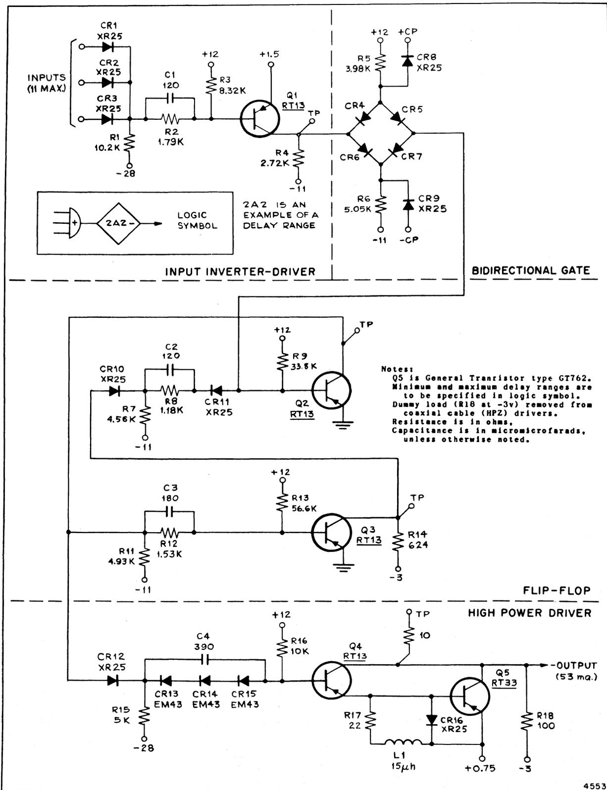
Figure 1-9. High-Power Pulseformer
