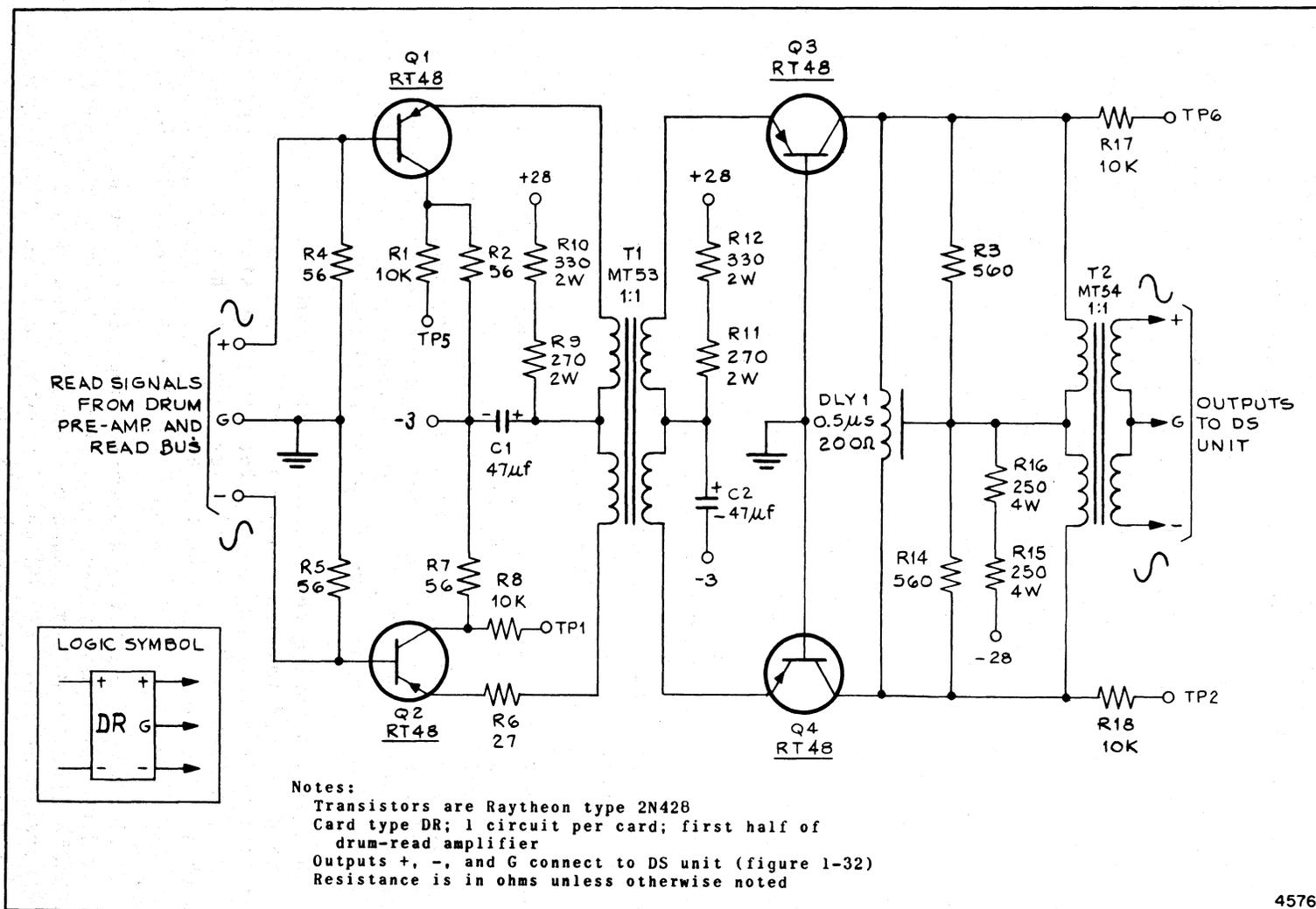
Figure 1-32. Drum Read Amplifier. Part 1
