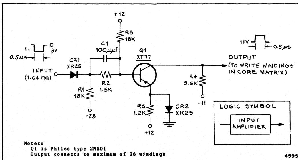
Figure 1-51. Input-Amplifier Circuit
