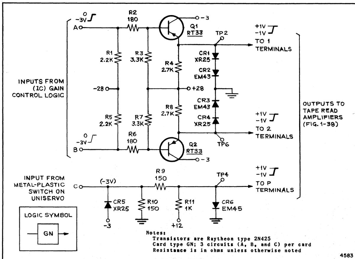
Figure 1-39. Gain-Control Network
