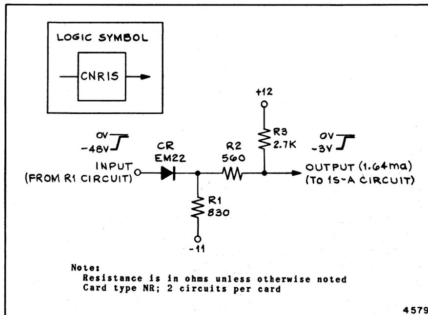
Figure 1-35. Type-CNR Coupling Circuit
