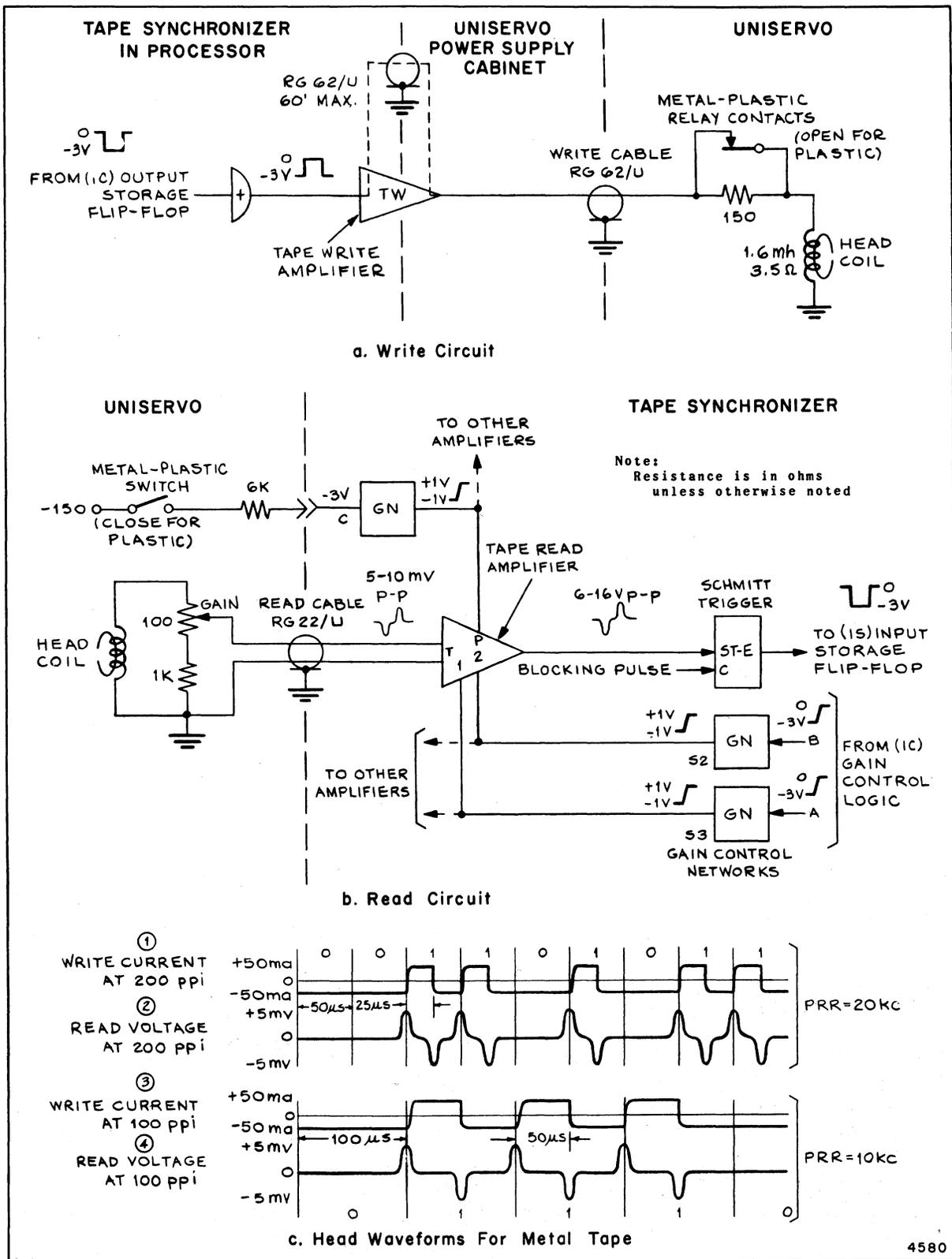
Figure 1-36. Tape Read-Write System (One Channel)
