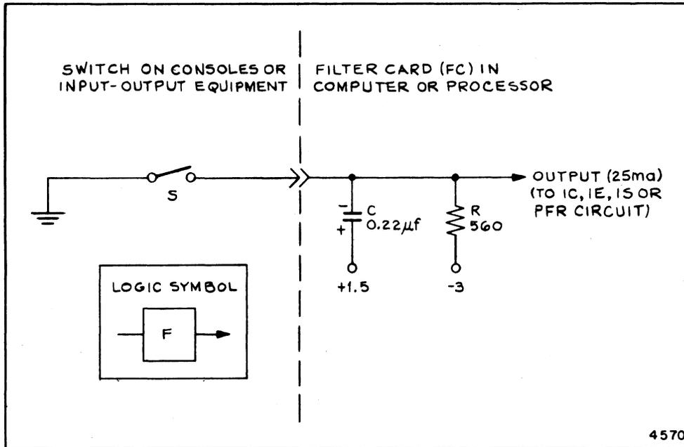
Figure 1-26. Type-F Filter Circuit
