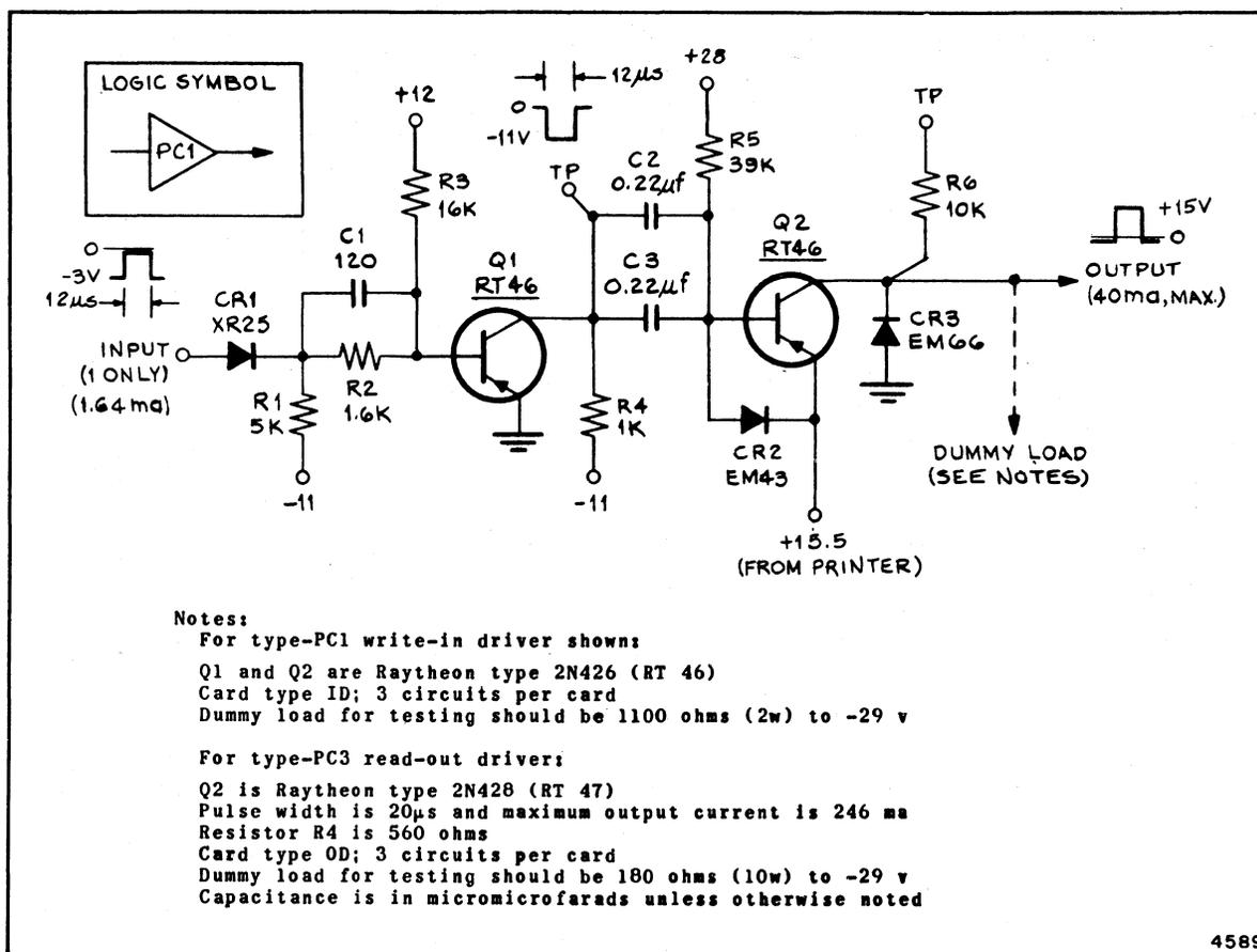
Figure 1-45. Type-PC1 and -PC3 Printer Core Drivers
