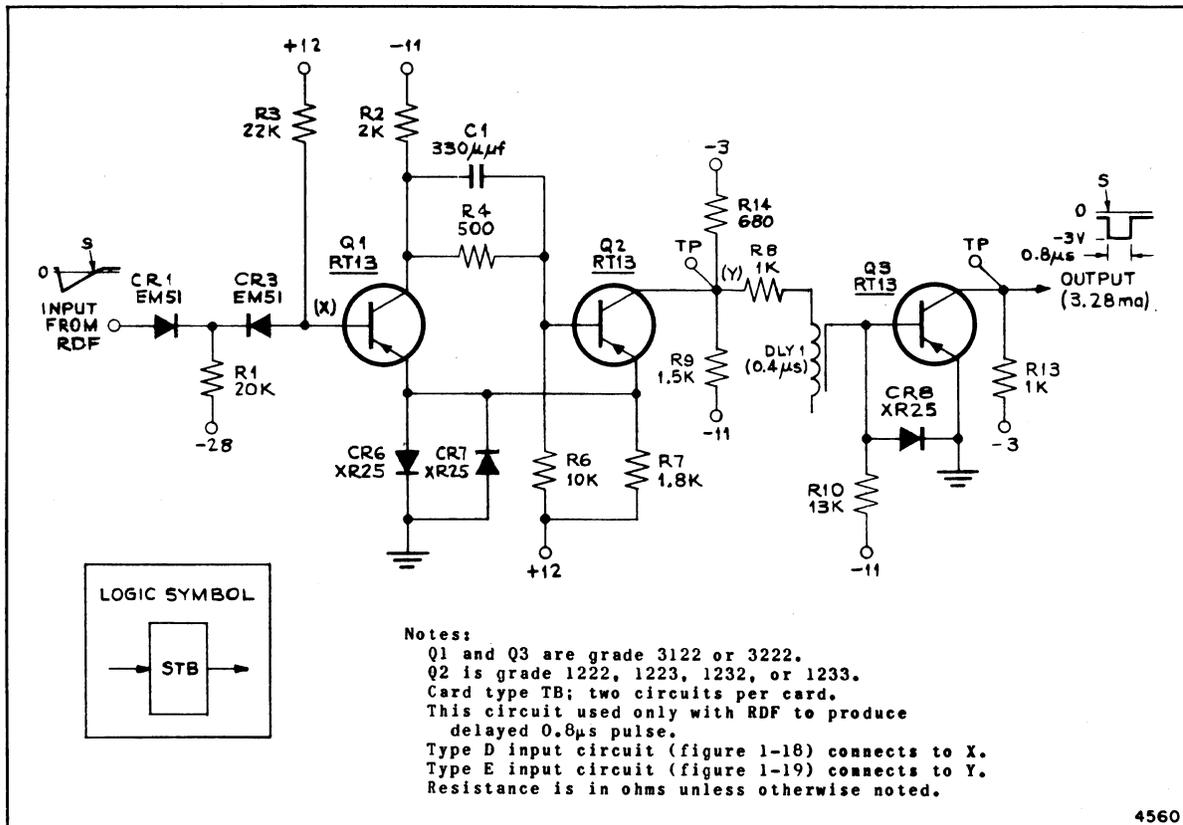
Figure 1-16. Type-ST-B Circuit
