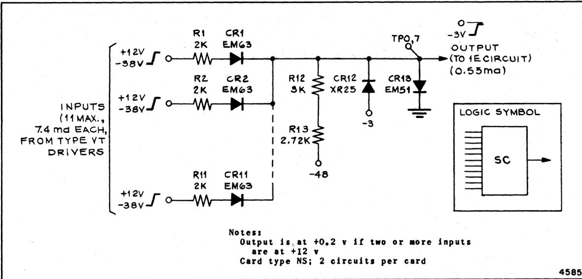
Figure 1-41. Tape-Selector Checker Circuit
