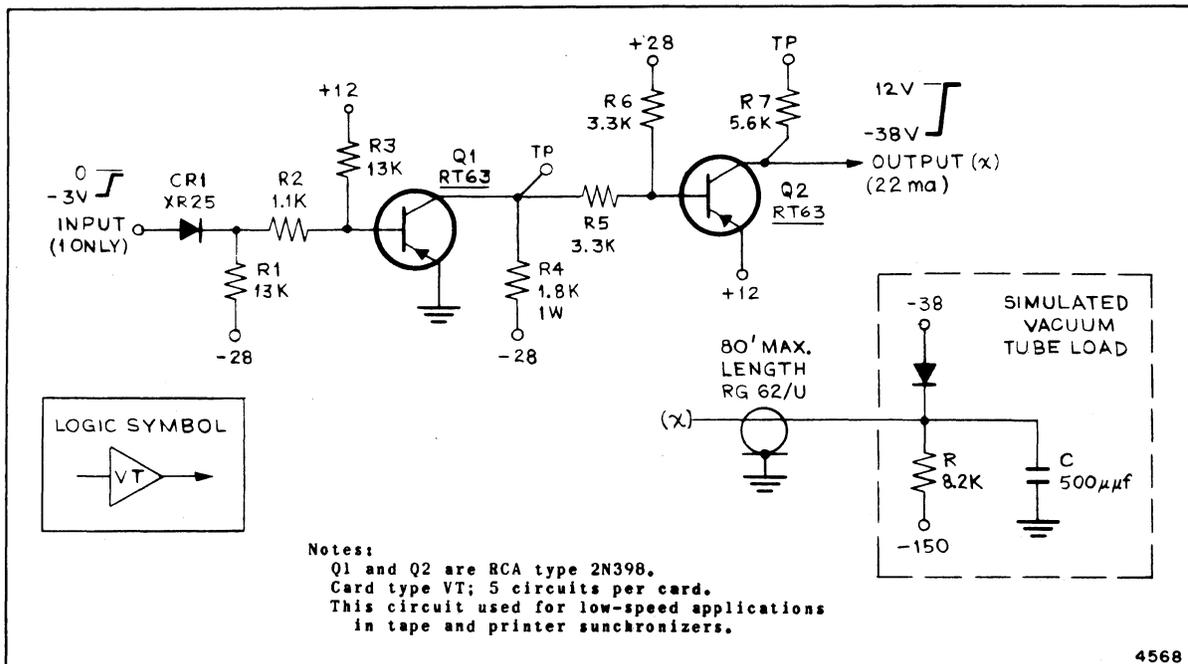
Figure 1-24. Type-VT Tube-Driver Circuit
