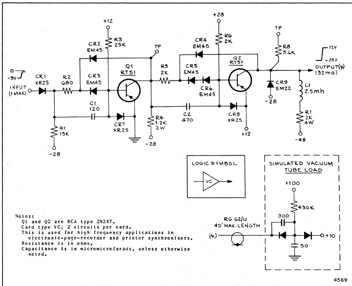
Figure 1-25. Type-VC Tube-Driver Circuit
