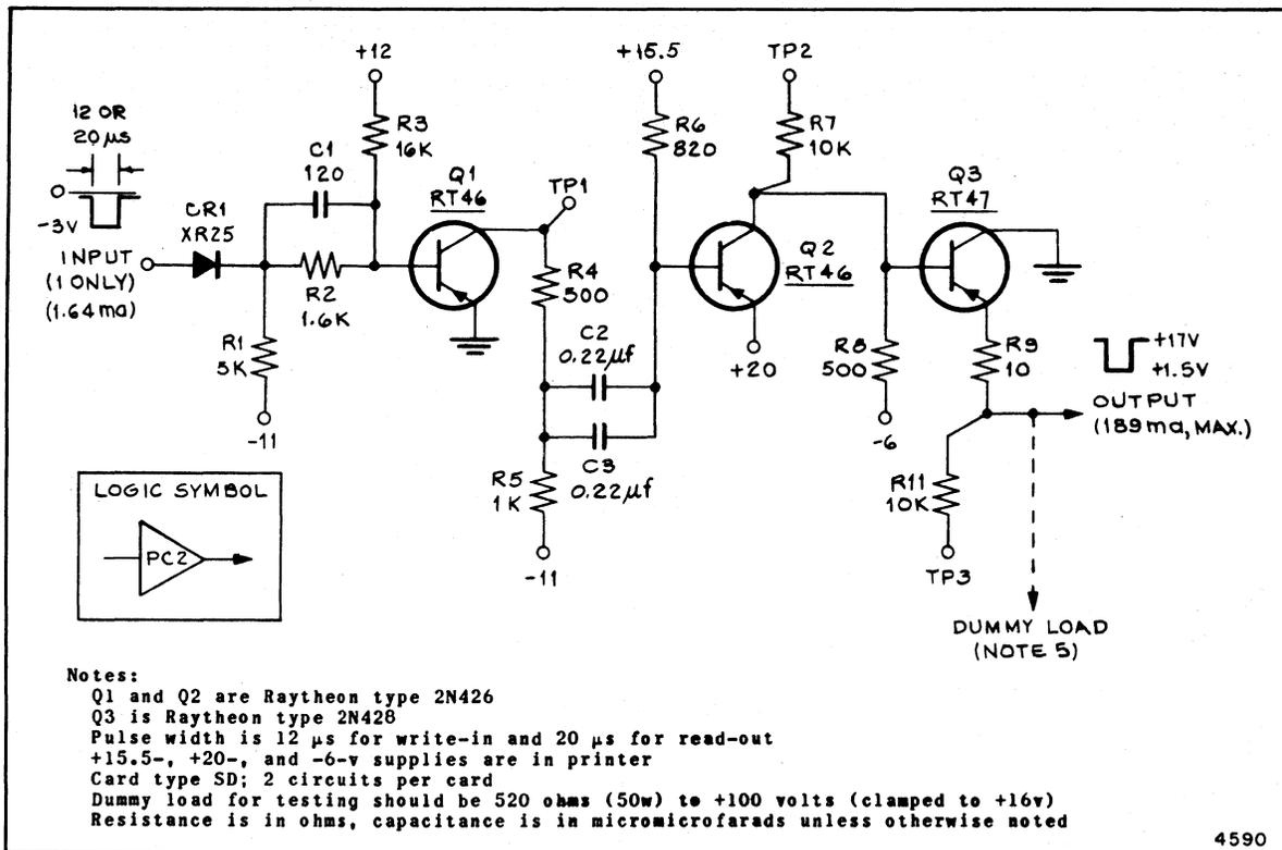
Figure 1-46. Type-PC2 Printer Core (Select) Driver
