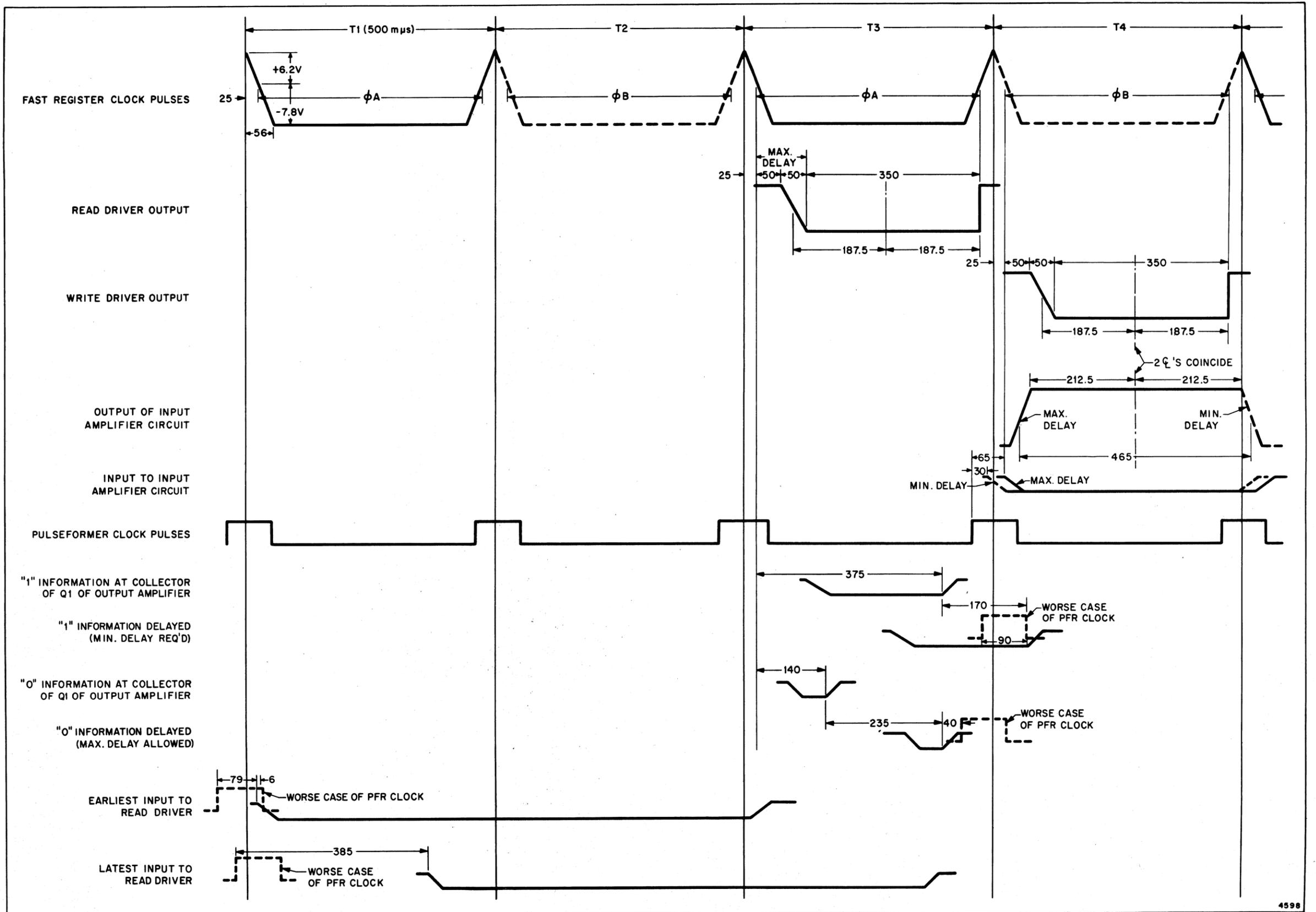
Figure 1-53. Timing Chart, A-B Register
