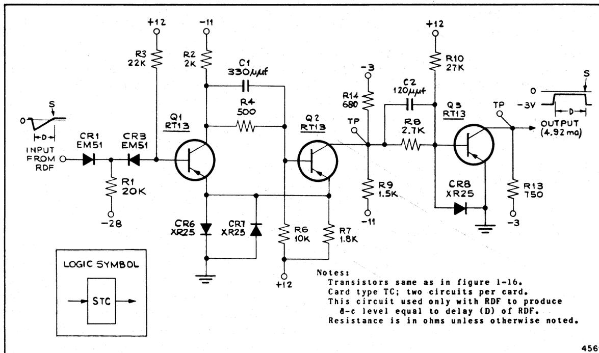
Figure 1-17. Type-ST-C Circuit
