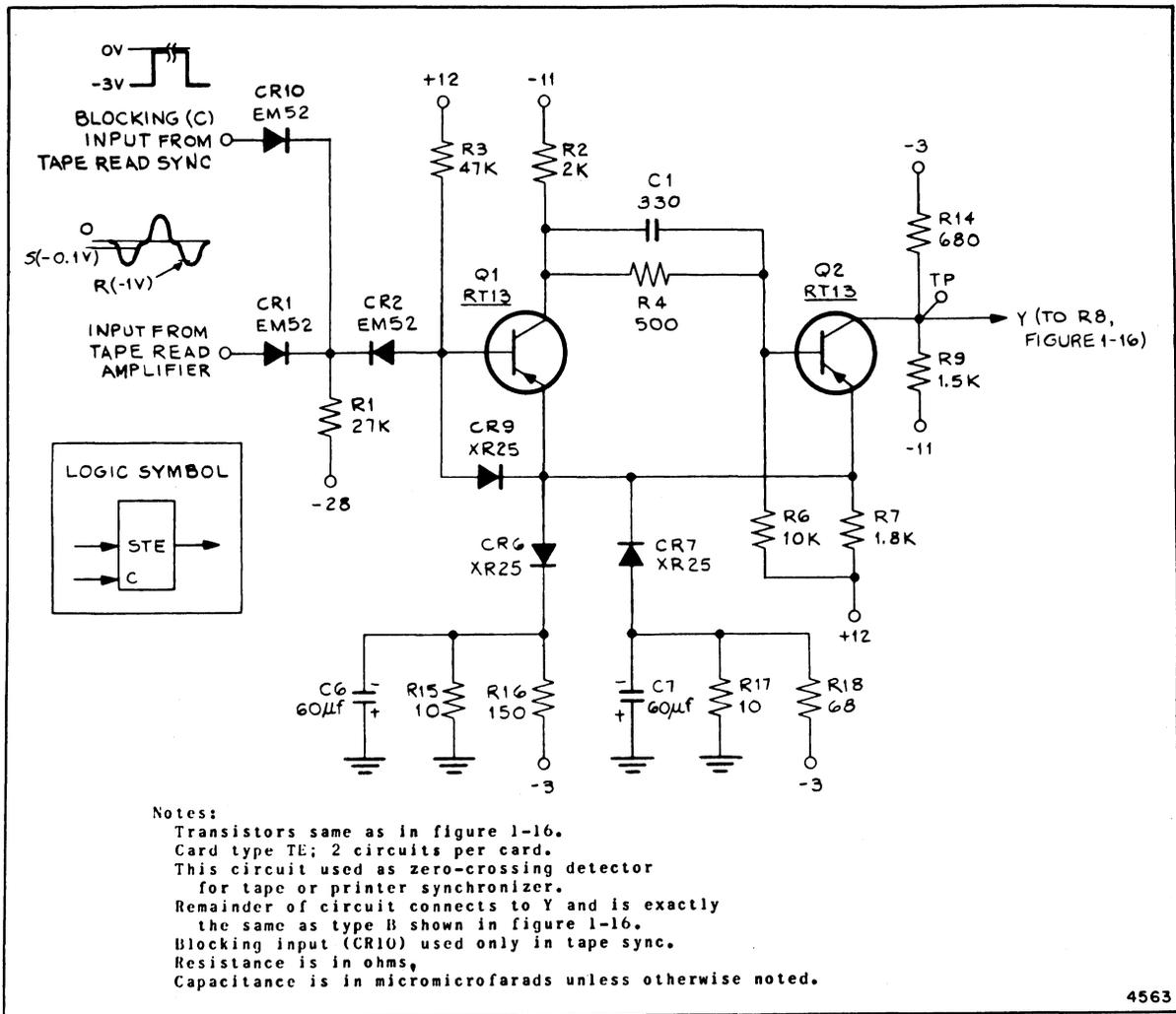
Figure 1-19. Type-ST-E Input Circuit
