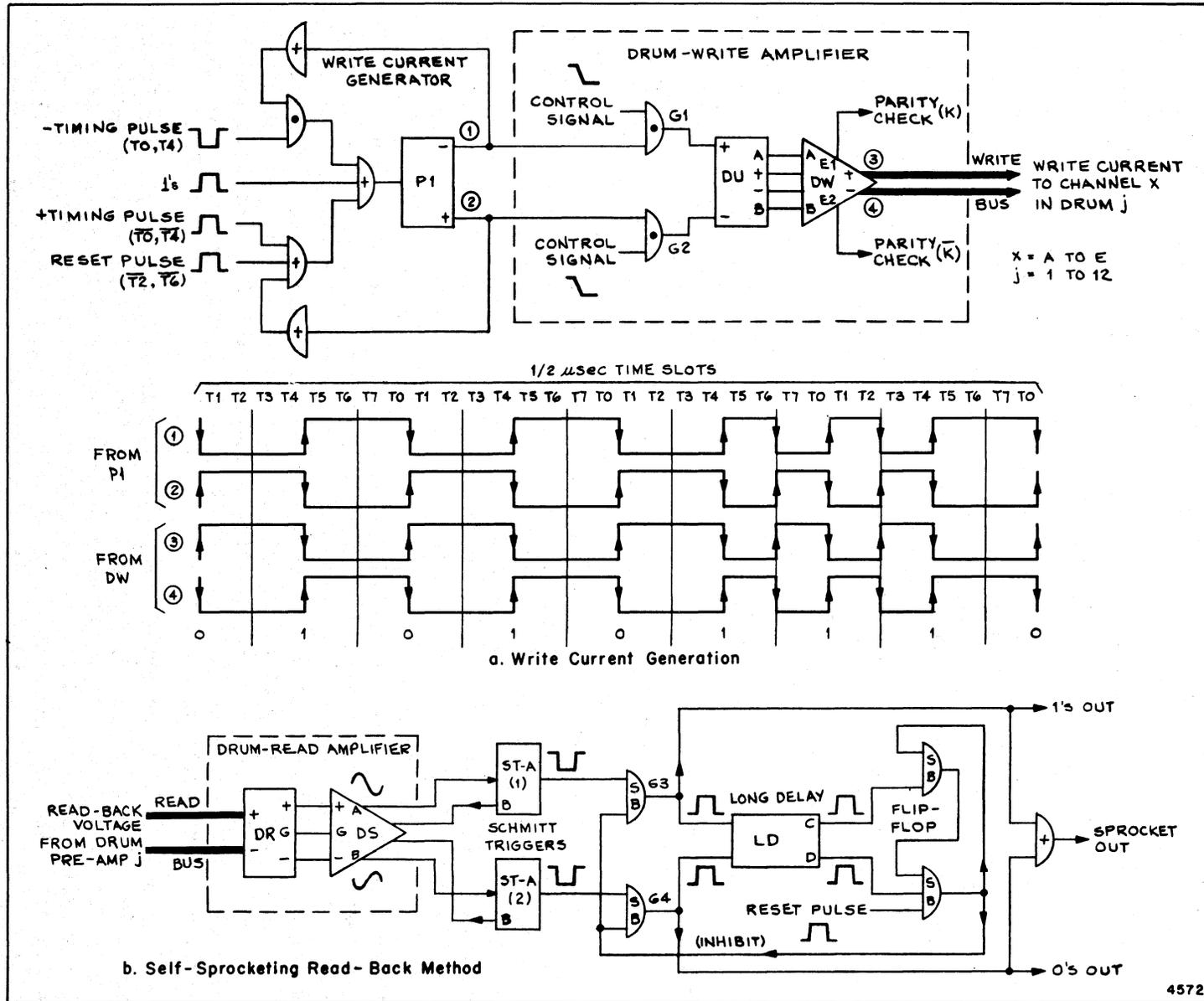
Figure 1-28. Drum Read-Write System (One Channel)
