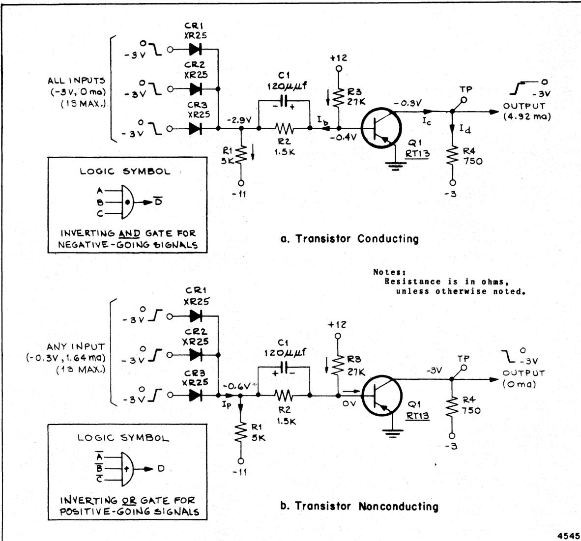
Figure 1-1. Type-1C Gate Inverter
