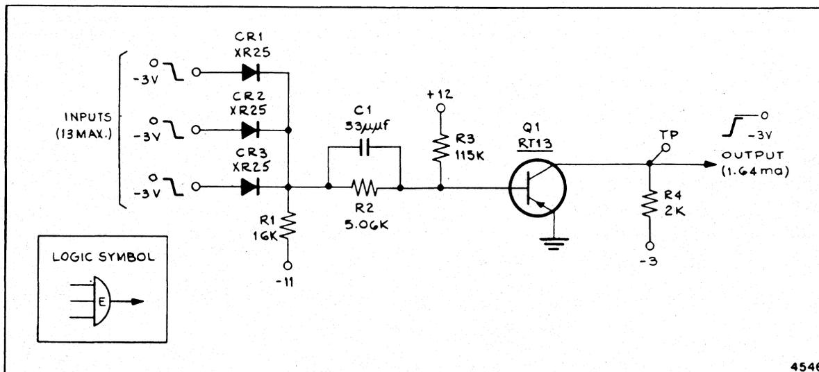
Figure 1-2. Type-1E Gate Inverter
