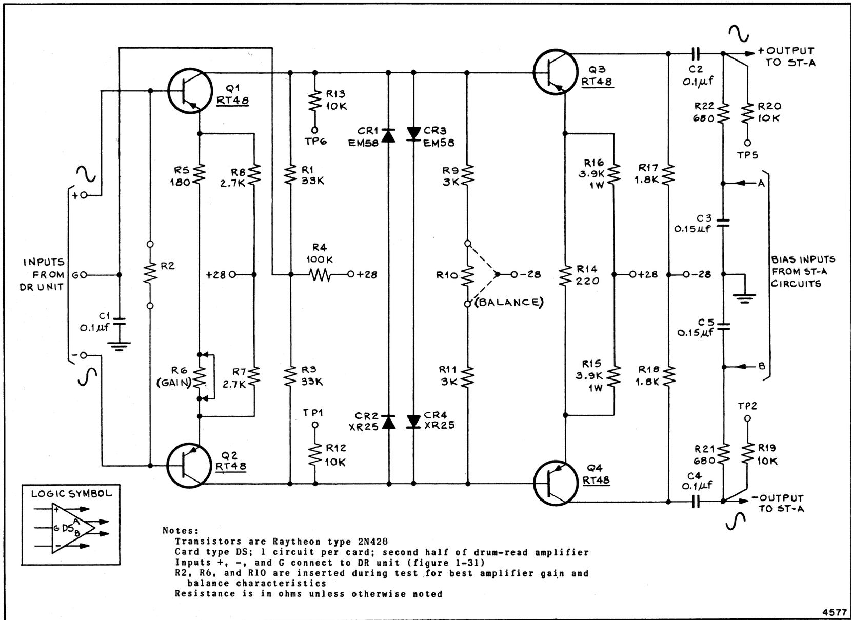
Figure 1-33. Drum Read Amplifier. Part 2
