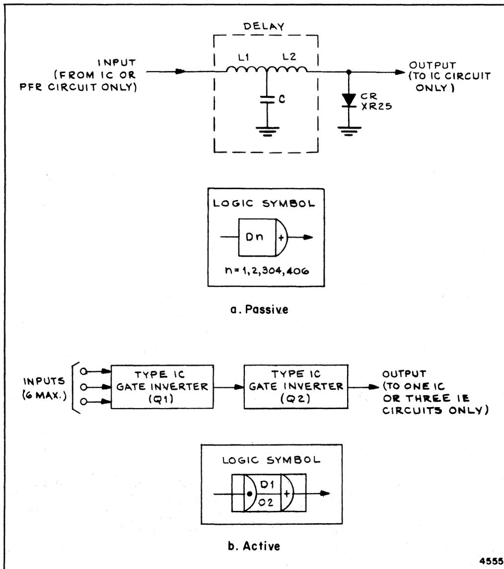
Figure 1-11. Delay Elements
