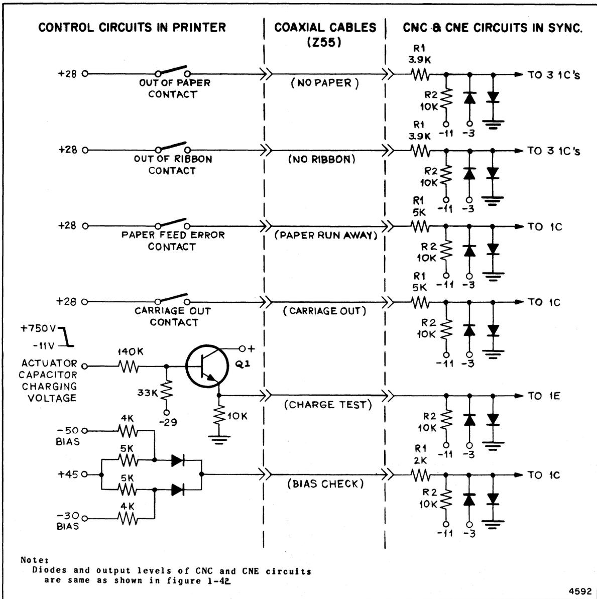
Figure 1-48. Line-Printer Coupling Networks
