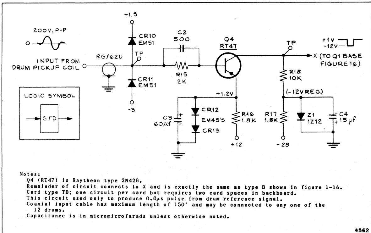
Figure 1-18. Type-ST-D Input Stage
