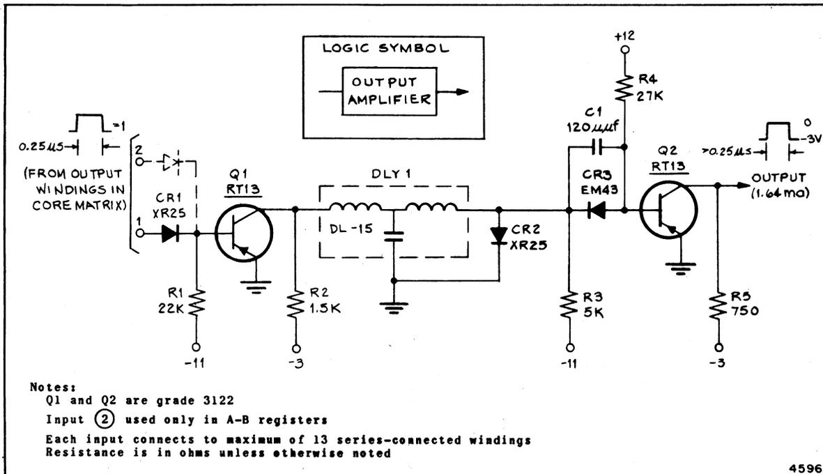
Figure 1-52. Output-Amplifier Circuit
