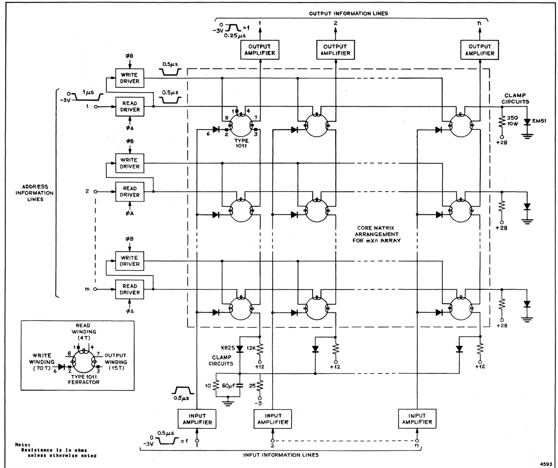
Figure 1-49. Fast-Register System for Parallel Operation
