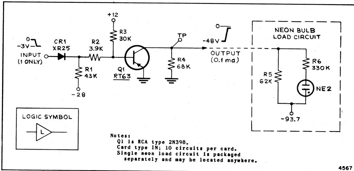
Figure 1-23. Type-L Indicator-Driver Circuit
