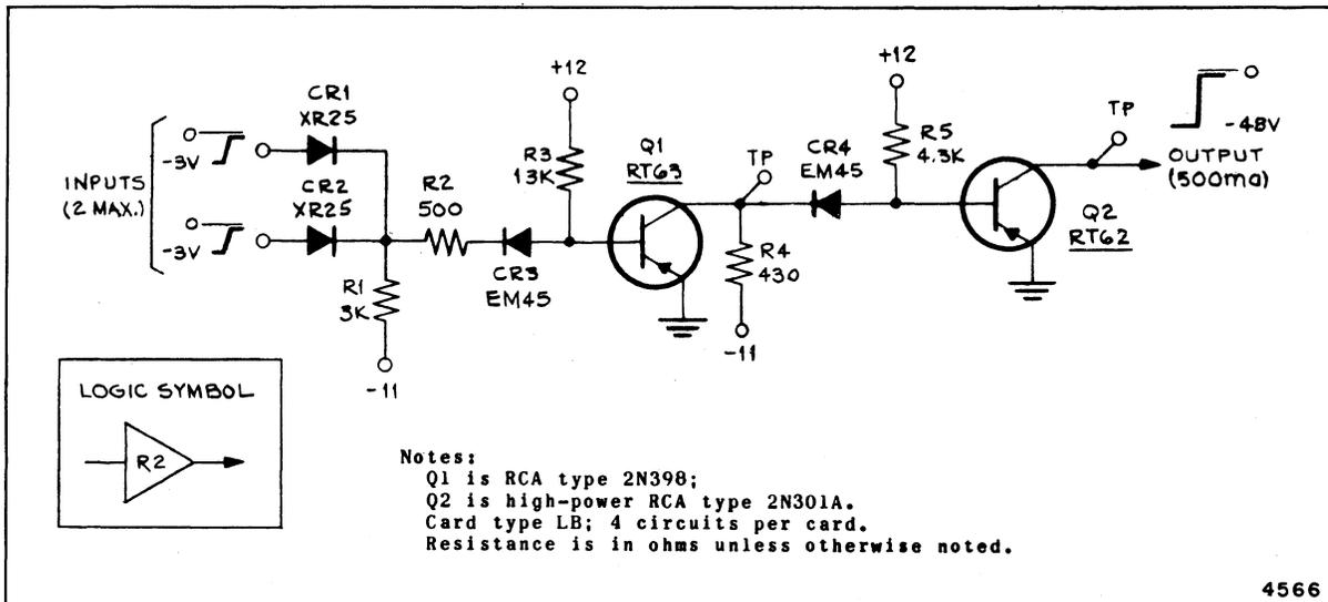
Figure 1-22. Type-R2 Low-Speed Driver Circuit
