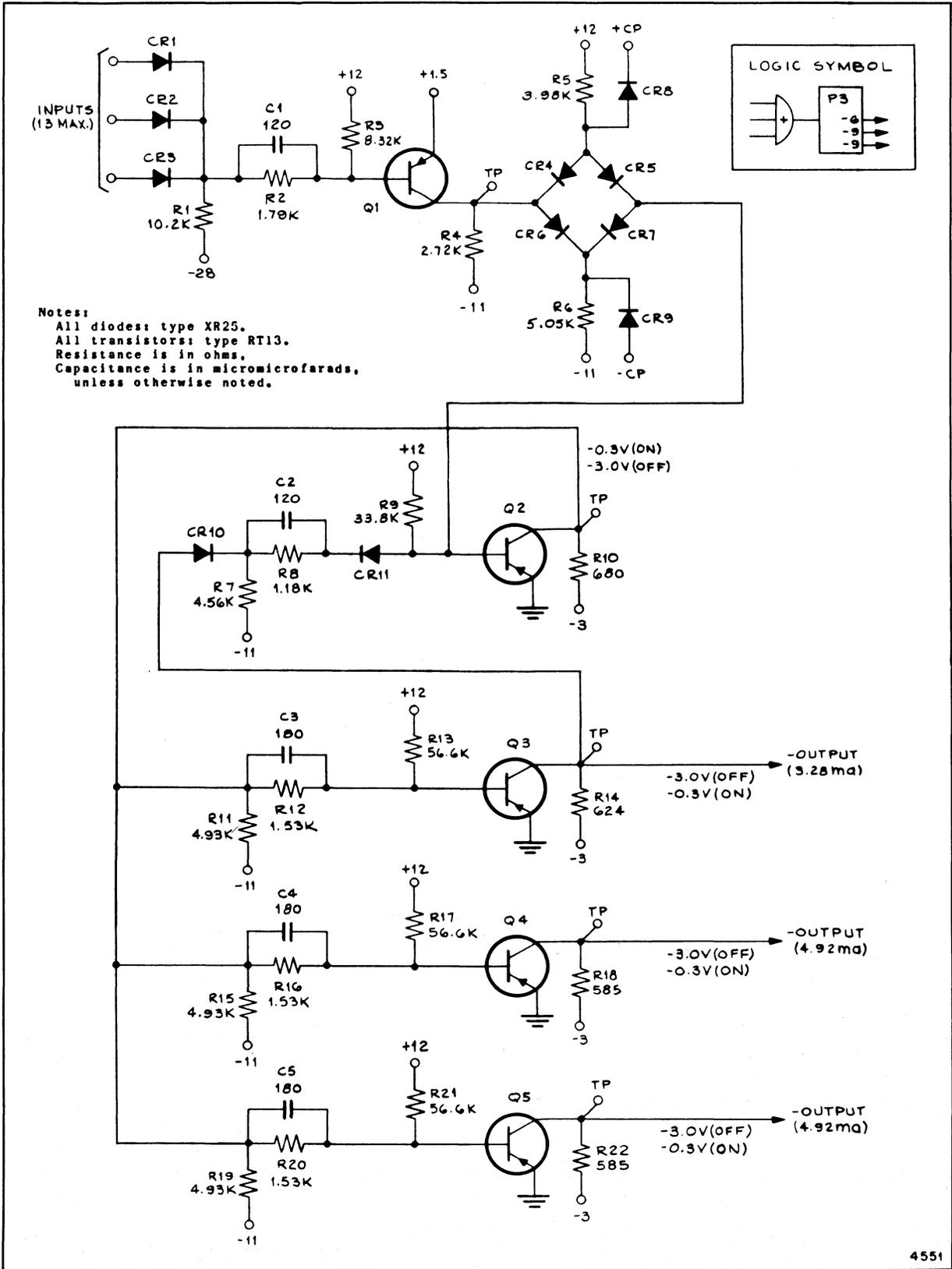
Figure 1-7. Type-P3 Pulseformer
