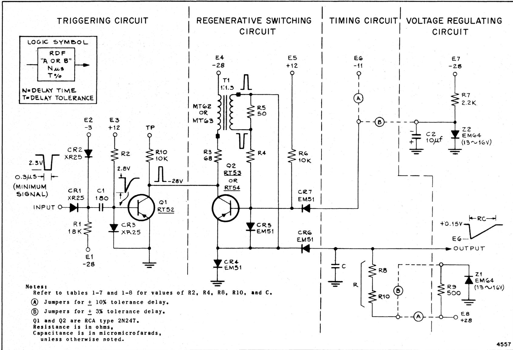
Figure 1-13. Retriggerable Delay Flop
