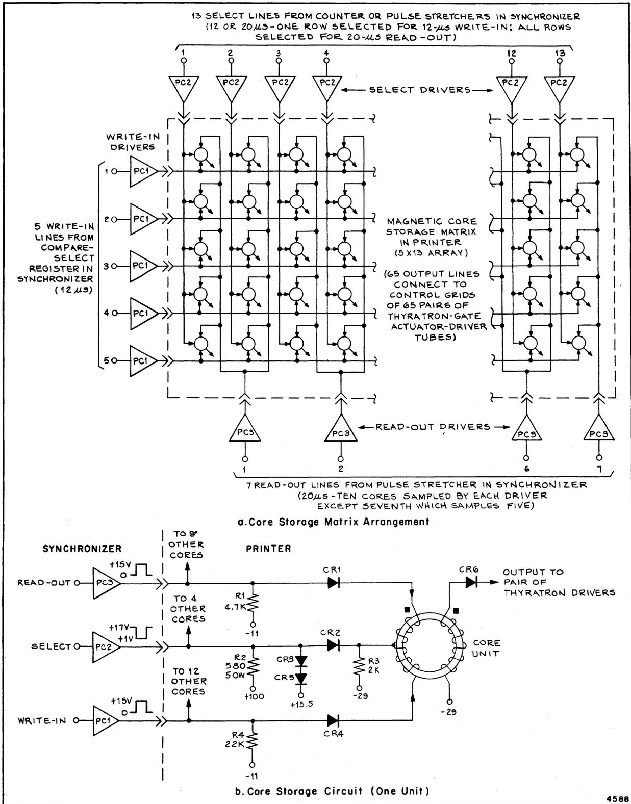
Figure 1-44. Line-Printer Core-Storage System
