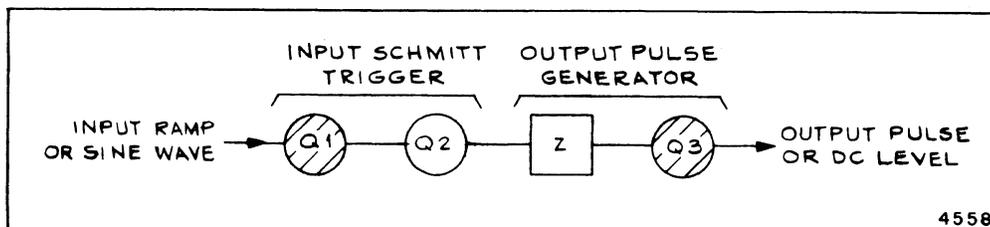
Figure 1-14. Schmitt Trigger, Block Diagram
