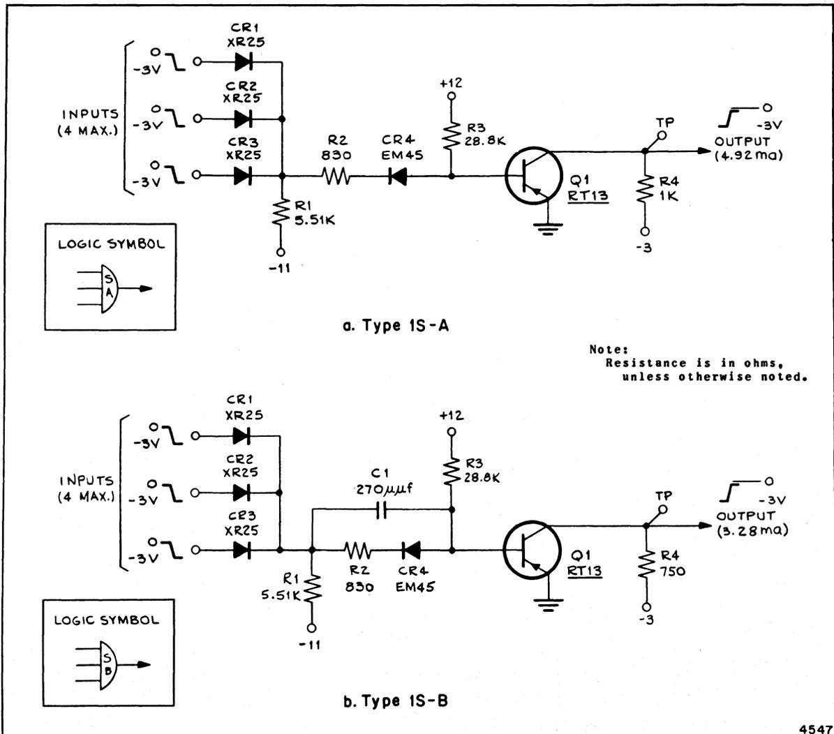
Figure 1-3. Type-1S Gate Inverter
