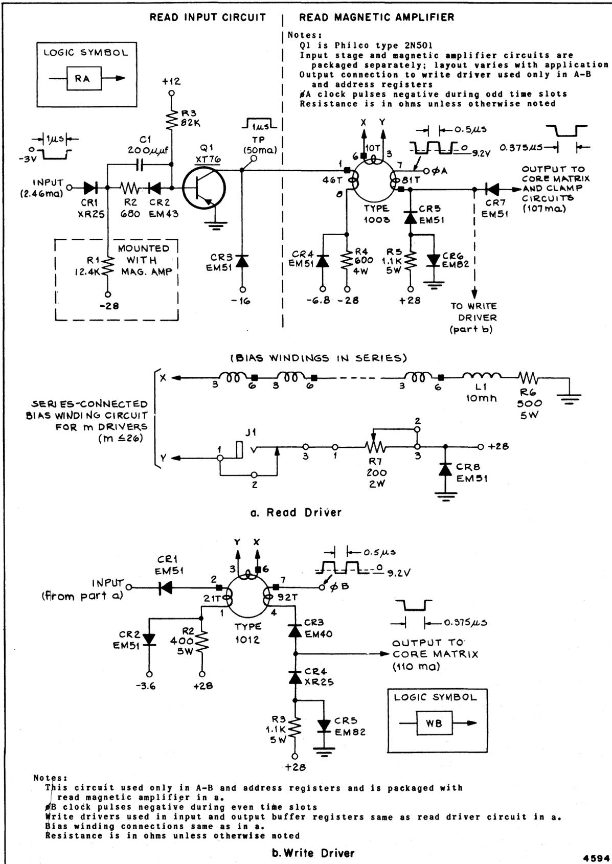
Figure 1-50. Read-Write Driver Circuits
