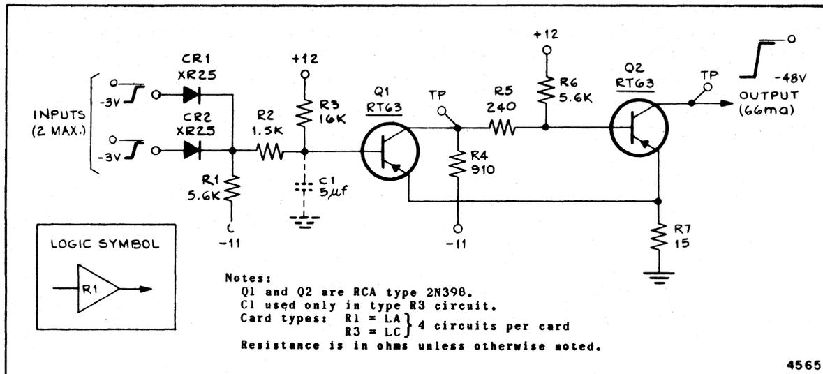
Figure 1-21. Type-R1 and -R3 Low-Speed Driver Circuit
