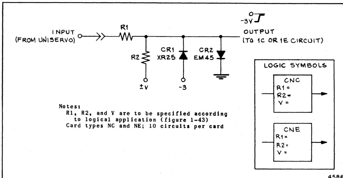
Figure 1-42. Type-CNC and -CNE Coupling Circuits
