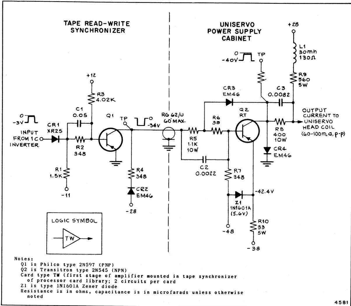
Figure 1-37. Tape Write Amplifier
