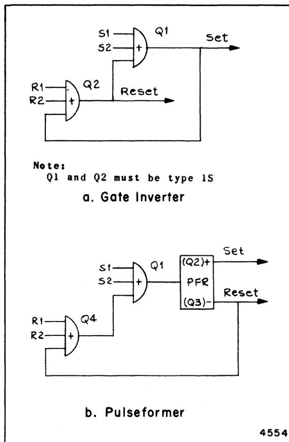
Figure 1-10. Flip-Flop Arrangements
