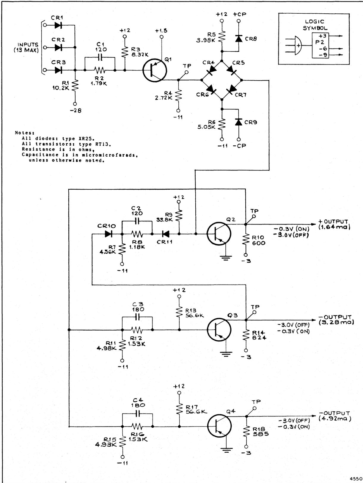
Figure 1-6. Type-P2 Pulseformer
