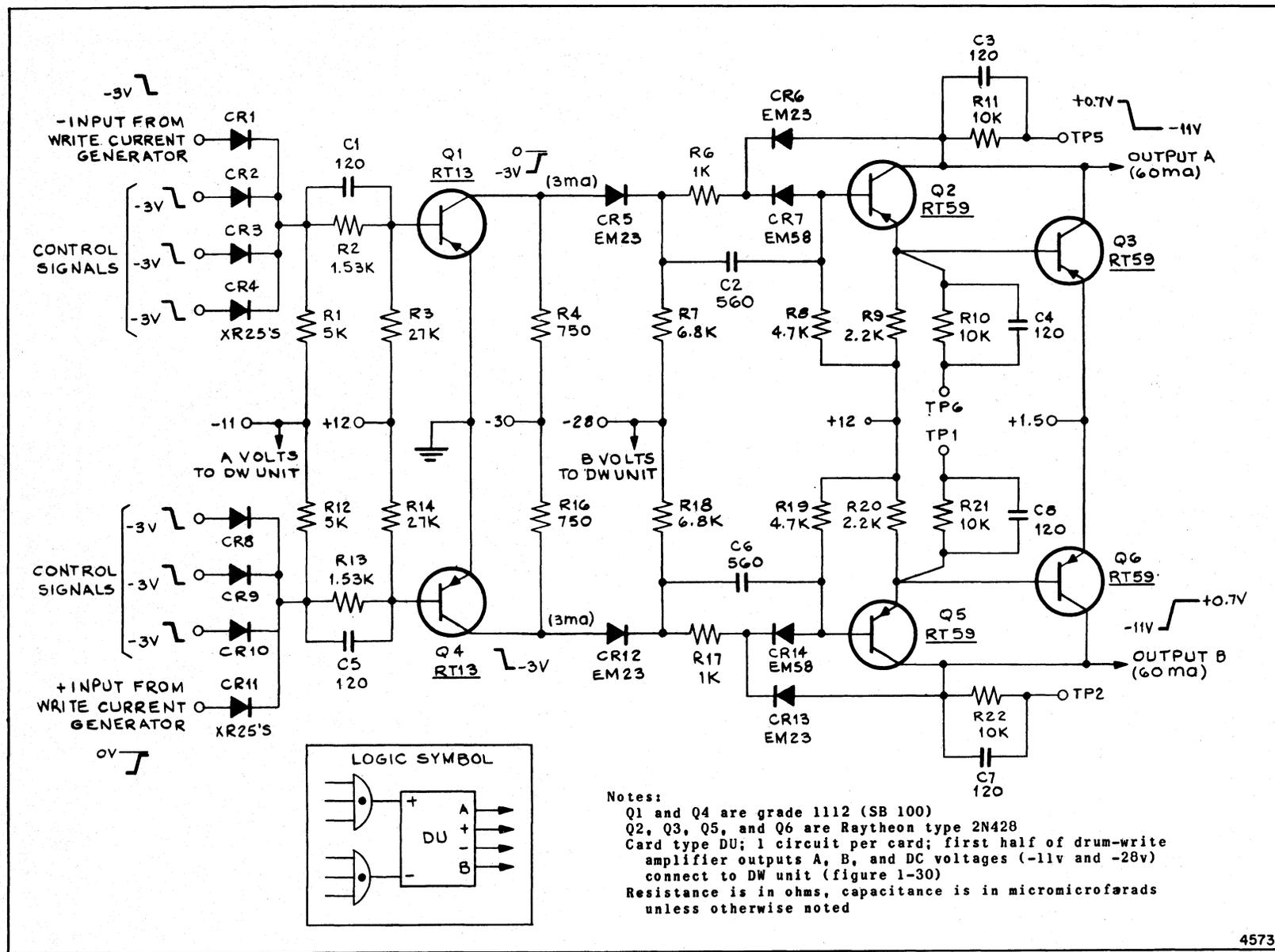
Figure 1-29. Drum Write Amplifier. Part 1
