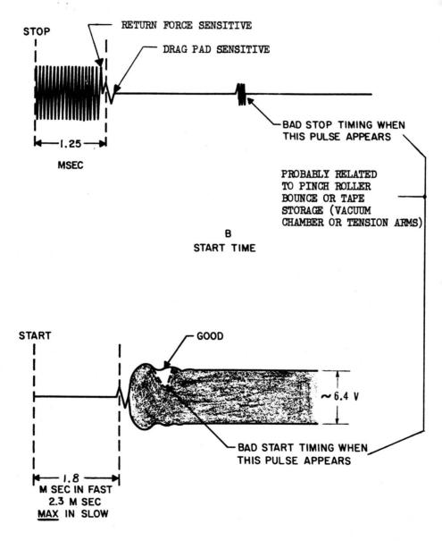
Figure 5. Transport Start-Stop Check Waveforms
