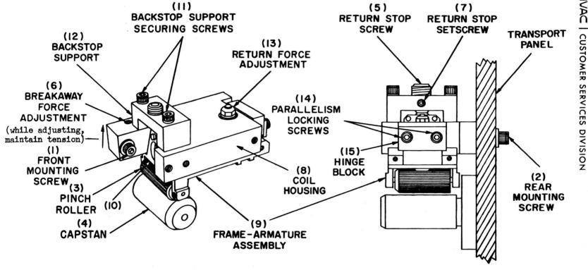
Figure 1. Solenoid Adjustments
