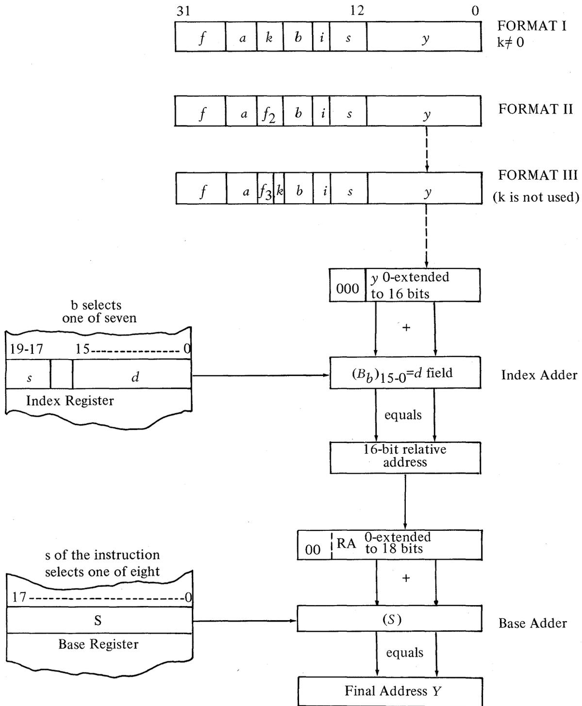
Figure 17. Direct-Address Generation
