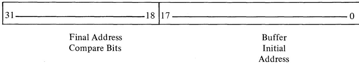
Figure 20. Main Memory Buffer Control Word Format
