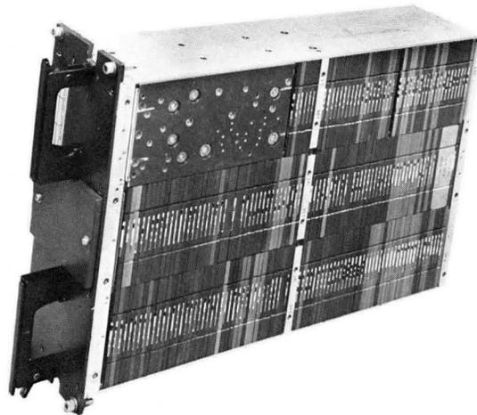
Figure 3. Central Processor (Card Side)
