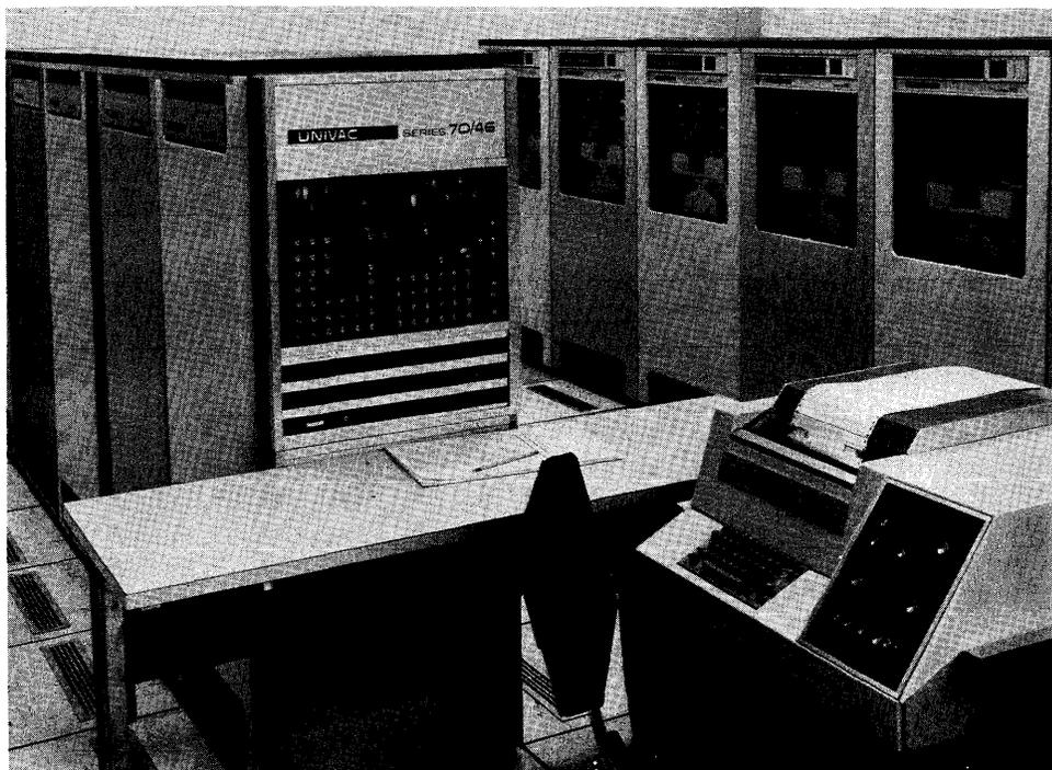
*The Series 70/46 Time-Sharing System is the virtual-memory version of the medium-scale 70/45 system. A 70/46 can service up to 48 users at remote terminals while concurrently processing up to 14 independent batch-mode jobs.*
