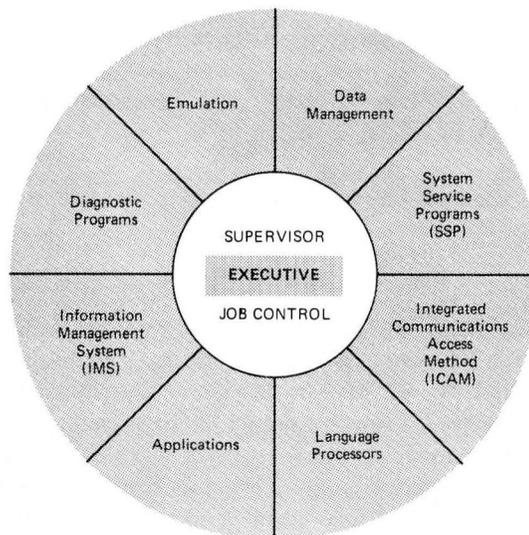
Figure 1-2. UNIVAC Operating System/3
