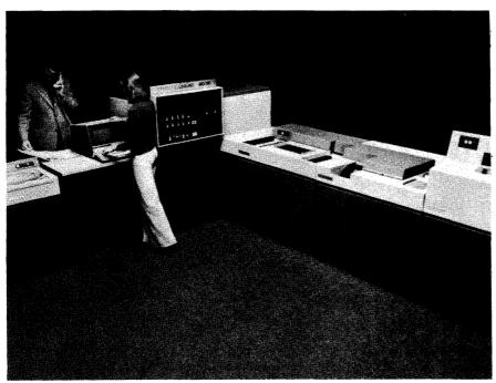
The basic UNIVAC 90/30 configuration includes a processor with 65K bytes of MOS storage, CRT system console, 500-cpm card reader, 500-lpm printer, and two 8416 Disk Drives with a total capacity of 57.8 million bytes. Also shown in the photo is an optional card punch.
