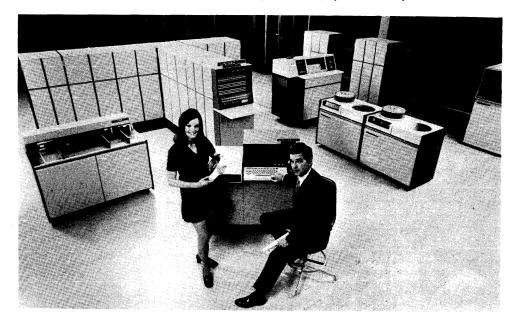
This view of a fairly small, disc-oriented UNIVAC 90/70 configuration shows CRT-equipped System Console in the foreground and the Central Processor at left rear.
