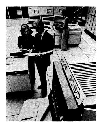
The UNIVAC 90/60, designed and priced to be an attractive alternative to the IBM 370/135, offers from 131K to 524K bytes of MOS main memory with a cycle time of 600 nanoseconds per 4-byte access. The same memory is used in the faster UNIVAC 90/70.
