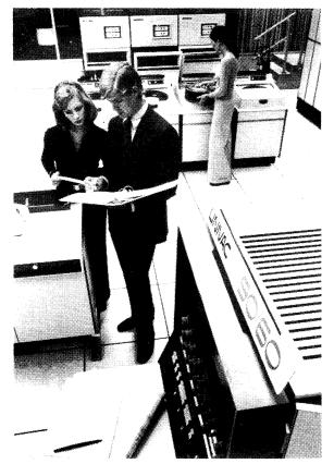
The UNIVAC 90/60, designed and priced to be an attractive alternative to the IBM 370/135, offers from 131K to 524K bytes of MOS main memory with a cycle time of 600 nanoseconds per 4-byte access. The same memory is used in the faster UNIVAC 90/70.
