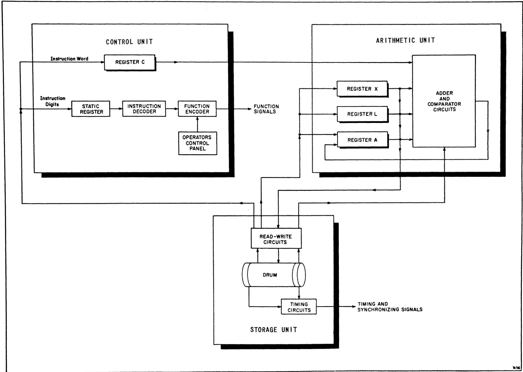
Figure 4. Central Processor Units
