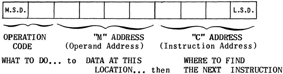
The "m" address is usually the address of a word in storage. The "operation code" tells the computer what to do with this word; and the "c" address is the storage location of the next instruction word. These fields may have different significance for some special instructions.
