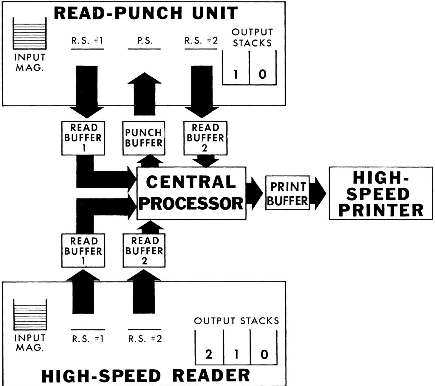
Figure 3. Buffer Operation
