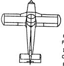
Aerotec 122 Uirapuru (Brazil) First Flight 1966 Data: Standard t-23 military version Cruising speed (Model A-122A) is 155mph Powered by 108hp Lycoming Engine Wing Span: 27 ft 10 3/4 in (8.5m)
