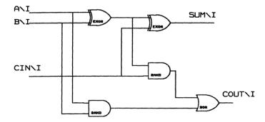
Figure 4-11. Full Adder Logic and Body Drawings
