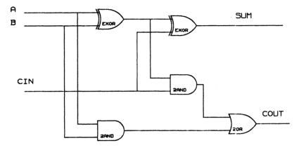
Figure 3-9. Sample Schematic with Signal Names
