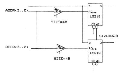
Figure 4-8. Manually Balancing Loads
