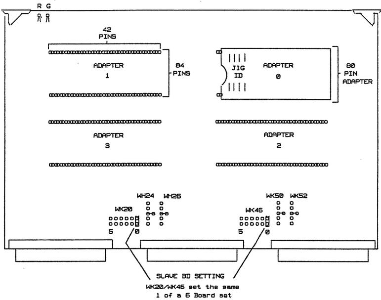
Figure 2-1. Realmodel DCM Jumper Locations
