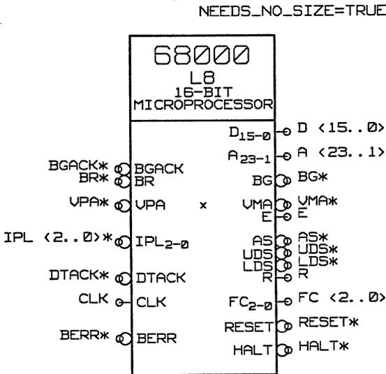
Figure 4-1. Typical .BODY Drawing
