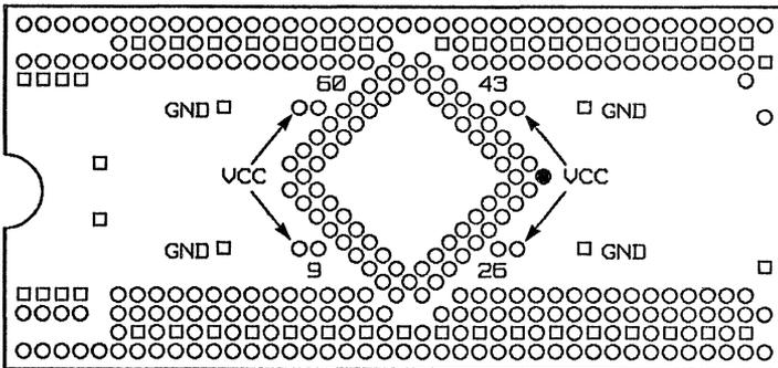
**Figure D-2. Power and Ground Wiring**
