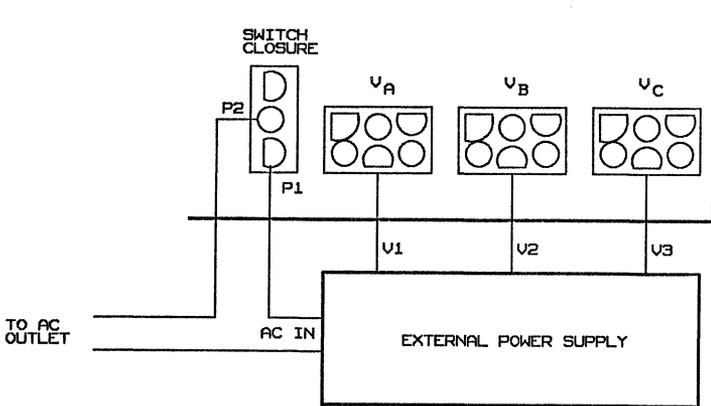
**Figure 2-5. Switch Closure Connector Wiring**
