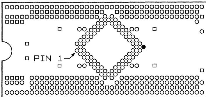
Figure D-1. 68-Pin LCC Personality Module
