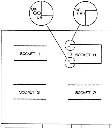
Figure 2-4. External Voltage Pins on DCM
