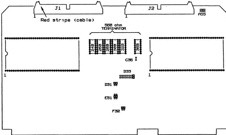
**Figure 2-2. Realchip DCM Jumper Locations**
