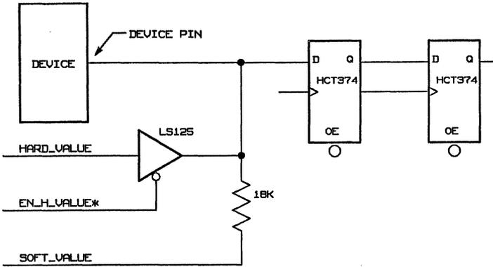
Figure 4-5. Sampling Circuit
