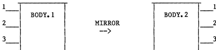
The MIRROR command should be used with caution, especially with bodies that have unmarked pins such as the Valid-supplied merge bodies. Reversal of the bit order can cause subtle, hard-to-find bugs within a design.
