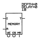
See the ValidSIM Reference Manual for information on the MEM\_STATE directive. The width of each word in the MEMORY primitive is determined by the SIZE property. The number of words is determined by the DEPTH property. The A (address) input has a size corresponding to the number of words. For example, a 256-word RAM has an A input width of eight.
