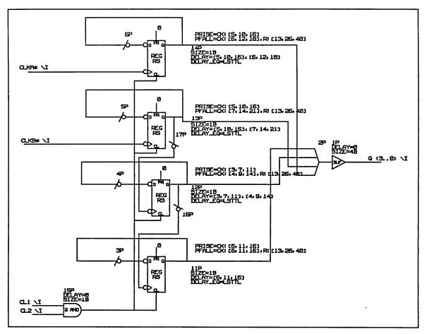
Figure 4-1. TTL 293 Simulation Model
