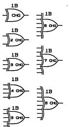
The most important non-standard primitive is the CHG (change) primitive. This primitive tells you whether an input signal is stable, changing, or unknown; frequently, this is all the information the Timing Verifier needs. When you add delay to the CHG primitive, you effectively model simple propagation delay through a component.
