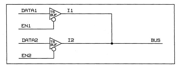
Figure 5–11. TS BUS Primitive
