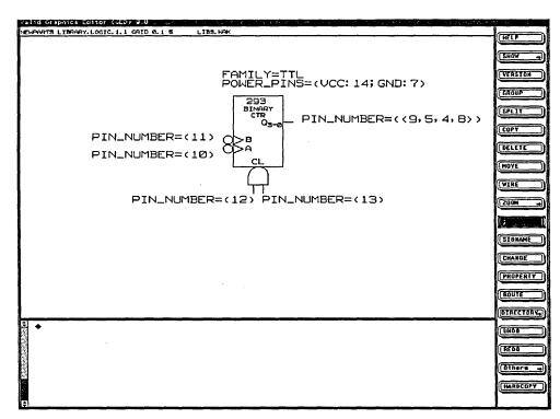
Figure 3-3. The TTL 293 Component with Pin Numbers
