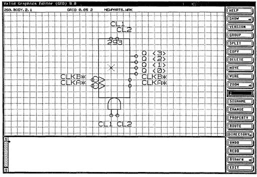
Figure 2-5. The TTL 293 Pin Names
