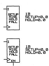
The SETUP HOLD primitive has an optional enable input that turns the checking on and off. If the enable input is any value other than zero, then checking is enabled. If checking is enabled any time during the rising edge of the clock input, then checking is performed for that edge.
