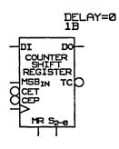
This component is very similar to the Fairchild 100K ECL component (F100136). The COUNTER SHIFT REGISTER primitive operates as either a modulo-16 up/down counter or as a four-bit bidirectional shift register. This primitive has seven inputs:
