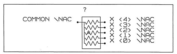
Figure 6-10. Version 2 of the RES5 SIP6 Resistor
