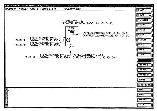
Figure 3-4. The TTL 293 Pin Loading Properties
