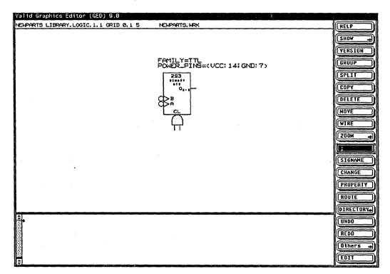
Figure 3-2. The TTL 293 Body Properties
