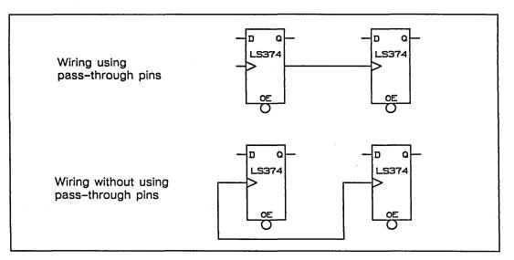
Figure 2-4. Using Pass-through Pins
