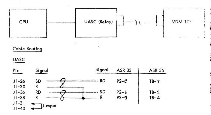
Note: The 2.0K and 2.7K resistors (RI3and RI4)must be in place when the UASC is interfaced to the TTYs as noted above.
