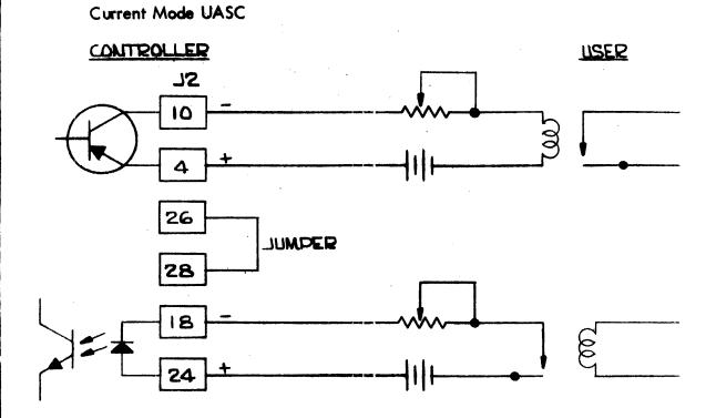
Note: As in 4.4.1.2, line battery can be one source if separate current limiting resistors are used.
