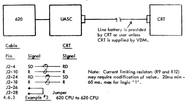
Hardwire controller to: bps = 1200, 2400, 4800, or 9600 bps. Set to 8 bits plus odd or even parity, 1 stop bit. Hook up cable as shown. See rate/distance table for max. length of cable.
