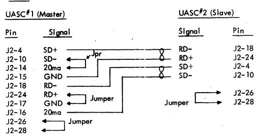
Note: Current limiting resistors R9 and R12 on both ends are shorted out for this application.
