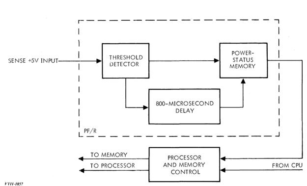
Figure 1-6. PF/R Block Diagram
