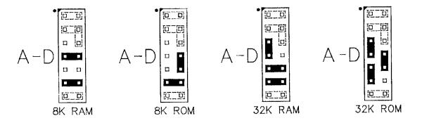
Figure 4-17. Chip Type Jumper Configurations
