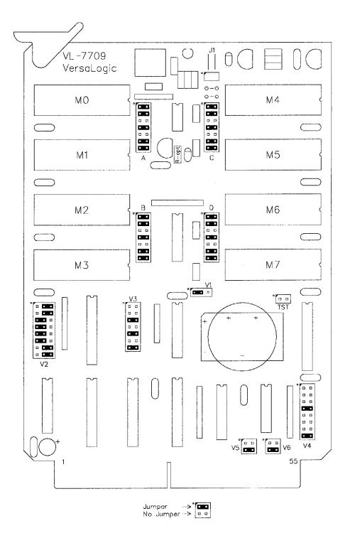
Figure 4-1. Jumper Block Locations
