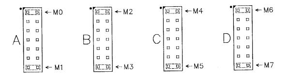
Figure 4-19. Memory Socket Enable Jumpers
