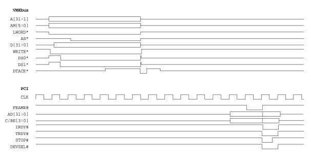
Figure C-8 Non-Block Decoupled Write Cycle - Universe II as VME Slave
