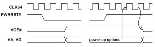
Figure 2-24 Power-up Options Timing
