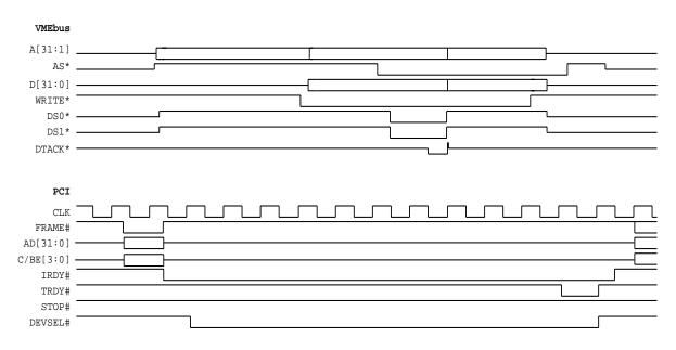
Figure C-7 Coupled Write Cycle - Universe II as VME Slave (bus parked at Universe II)
