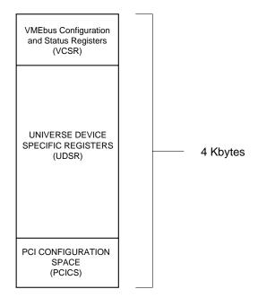
Figure 2-18 Universe II Control and Status Register Space
