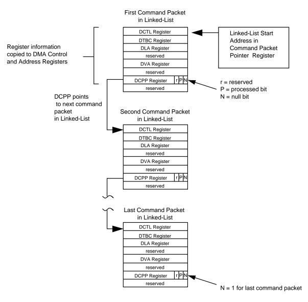
Figure 2-16 Command Packet Structure and Linked List Operation
