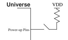
Figure D-2 Power-up Configuration Using Passive Pull-ups
