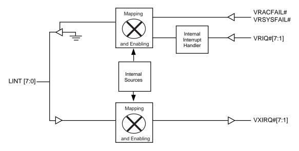
Figure 2-12 Universe Interrupt Circuitry
