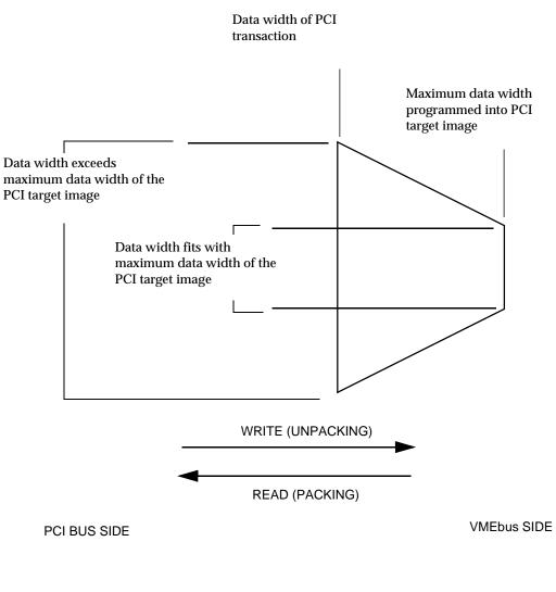
Figure 2-4 Influence of Transaction Data Width and Target Image Data Width on Data Packing/Unpacking
