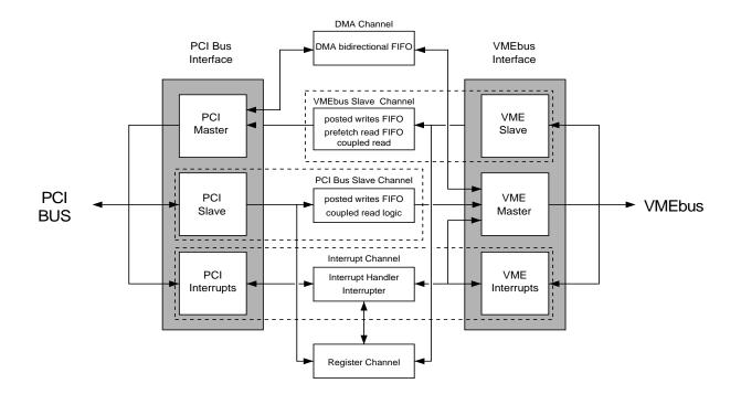
Figure 2-3 Architectural Diagram for the Universe II
