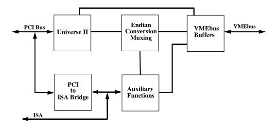
Figure 2-1 Universe II-Based PCI-to-VMEbus Interface
