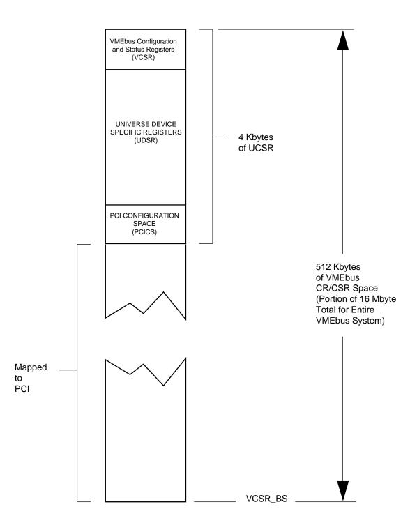
Figure 2-21 UCSR Access in VMEbus CR/CSR Space
