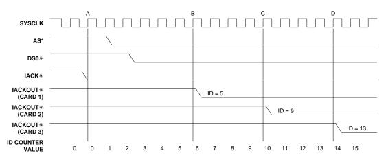
Figure 2-6 Timing for Auto-ID Cycle
