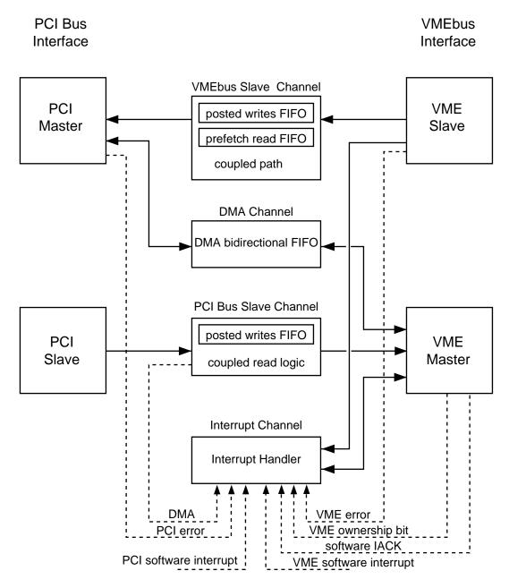
Figure 2-14 Sources of Internal Interrupts
