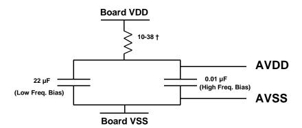
Figure D-5 Noise Filter Scheme
