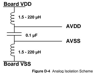
Figure D-4 Analog Isolation Scheme
