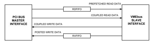
Figure 2-5 VMEbus Slave Channel Dataflow
