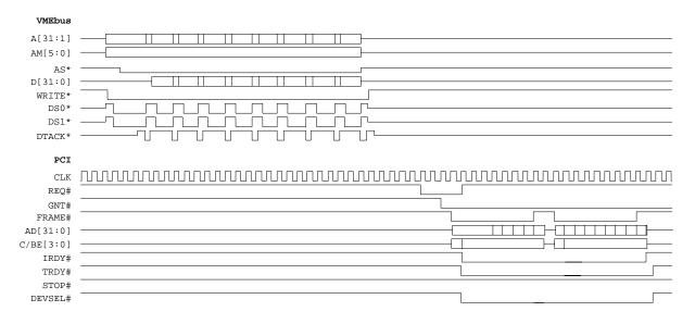
Figure C-10 MBLT Decoupled Write Cycle - Universe II as VME Slave
