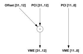
Figure 2-10 Address Translation Mechanism for PCI Bus to VMEbus Transfers
