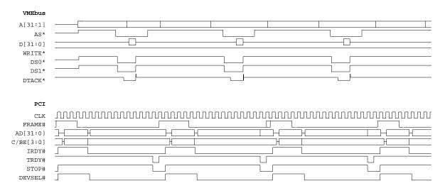
Figure C-2 Several Coupled Read Cycles - Universe II as VME Master
