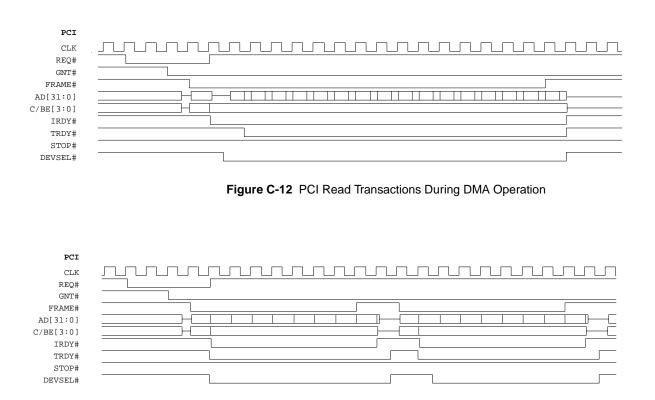
Figure C-13 Multiple PCI Read Transactions During DMA Operation
