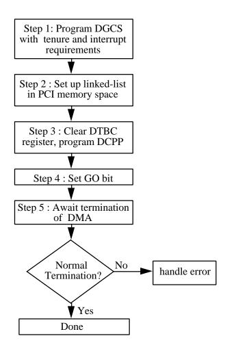
Figure 2-17 DMA Linked List Operation
