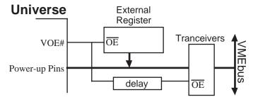
Figure D-3 Power-up Configuration Using Active Circuitry
