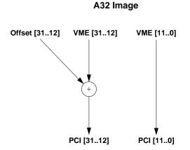
Figure 2-9 Address Translation Mechanism for VMEbus-to-PCI Bus Transfers
