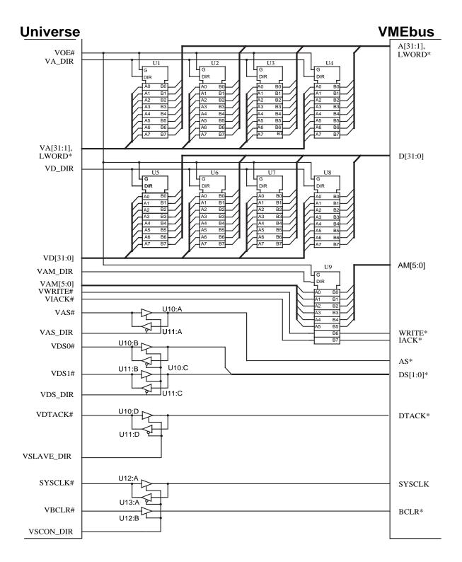
Figure D-1 Universe II Connections to the VMEbus Through TTL Buffers (continued)
