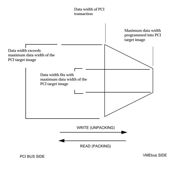
Figure 2-8 Influence of Transaction Data Width and Target Image Data Width on Data Packing/Unpacking
