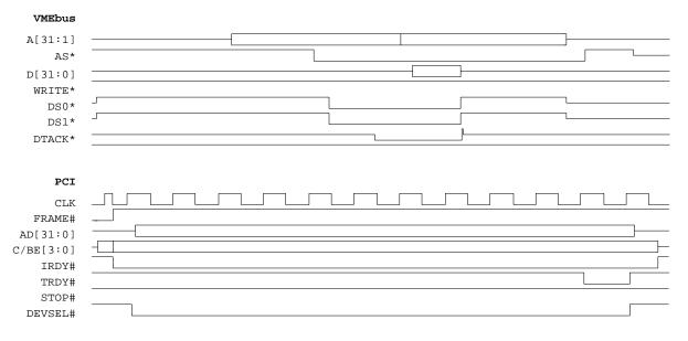
Figure C-6 Coupled Read Cycle - Universe II as VME Slave
