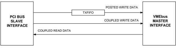
Figure 2-7 PCI Bus Target Channel Dataflow
