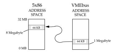
Figure 4-9 Remap of VMEbus Space to 5x86 Space
