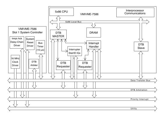
Figure 4-1 VMIVME-7586 VMEbus Functions
