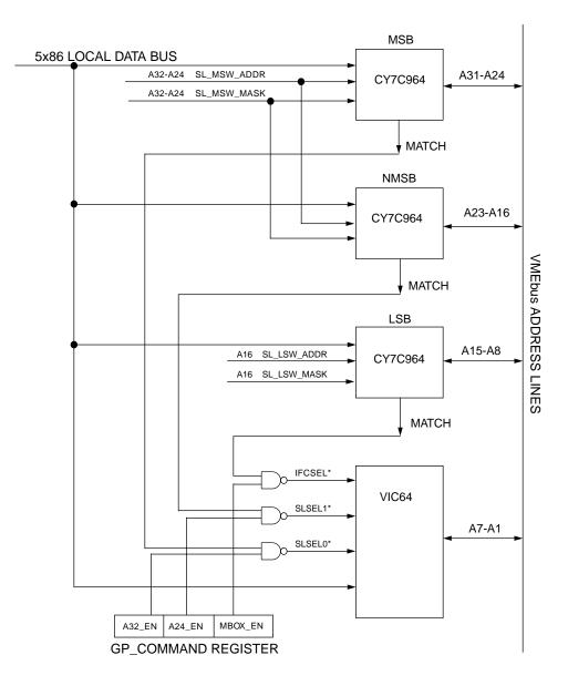
Figure 4-7 VMEbus Slave Interface
