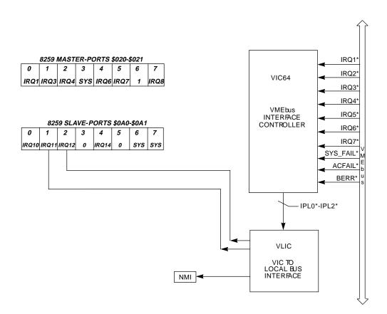
Figure 3-1 Connections Between the PC Interrupt Logic Controller and the VMEbus
