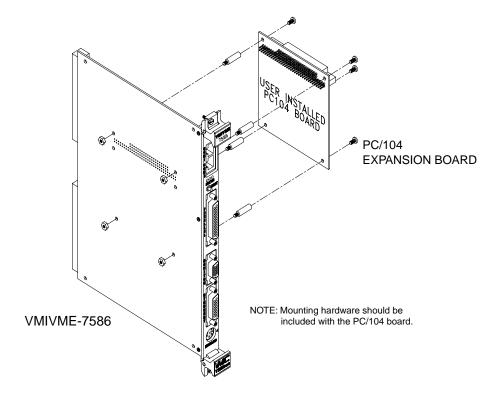
Figure 2-3 PC/104 Mechanical Connection
