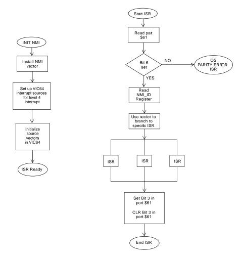
Figure 4-13 Flowchart for NMI Interrupt Processing
