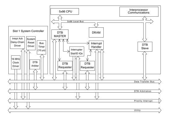
Figure 1-3 VMIVME-7586 VMEbus Functions
