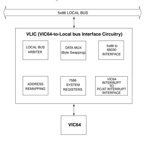
Figure 4-3 VLIC Block Diagram
