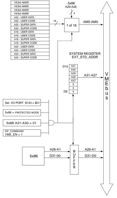
Figure 4-6 128 Mbyte Protected Mode VMEbus Access
