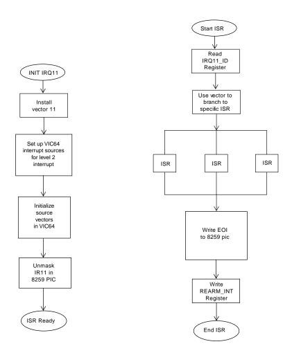
Figure 4-12 Flowchart for Non-NMI Interrupt Processing for IRQ11
