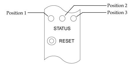
Figure 2-2 LED Position on the Front Panel
