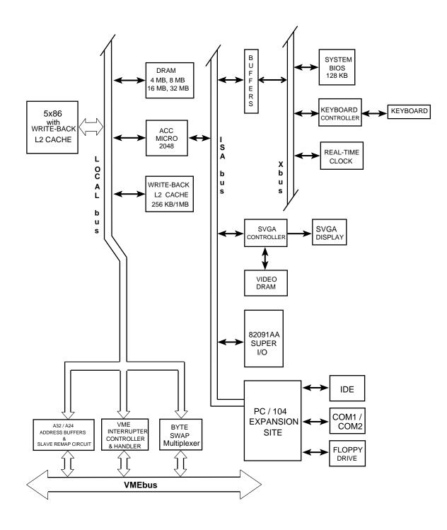
Figure 1-2 VMIVME-7586 Partial Block Diagram
