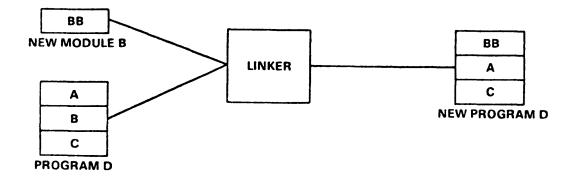
Figure 3-2. Replacement of a Module in a Linked Program
