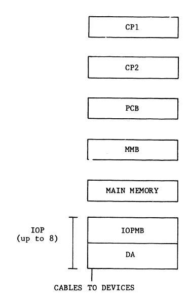
Figure 1-2 Printed Circuit Boards in a VS 100
