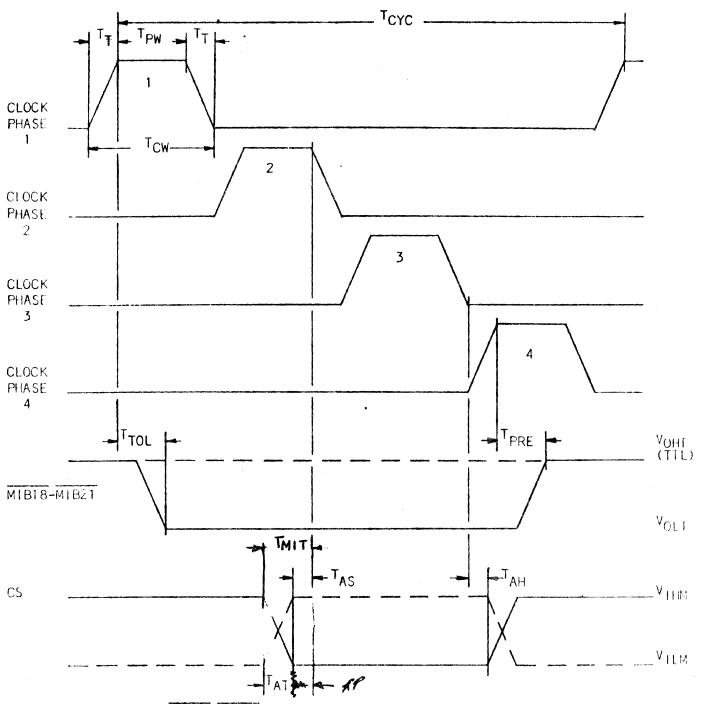
NOTE: TIL outputs (MIB18-MIB21) are unconditionally driven high at Ø4 and conditionally driven low at Ø1. This conditional low will be valid until the next Ø4.
