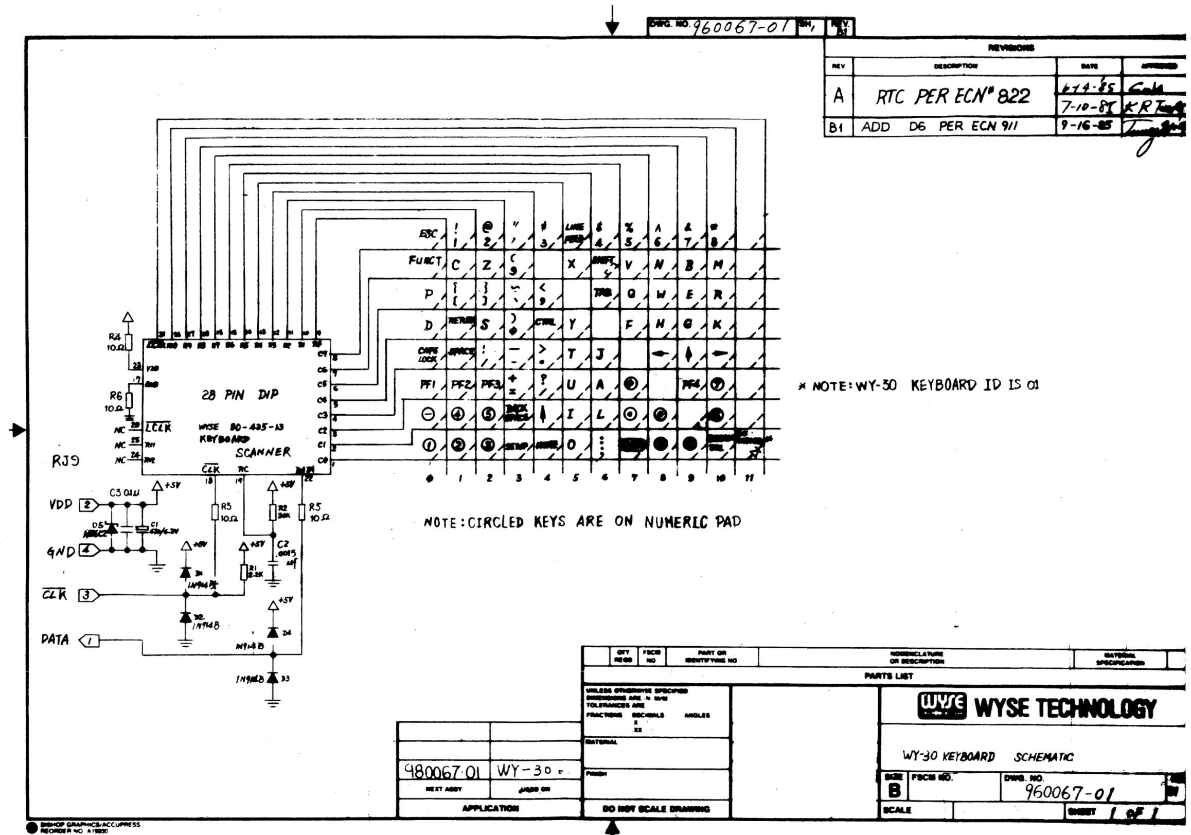
Figure 7-2 Terminal PCB Schematic (Logic)
