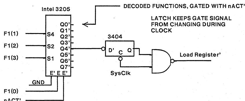
**Figure 3. FUNCTION DECODE****BUS(00)-BUS(15)**
