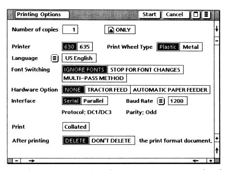
**3. Select** [630/635] for the Printer option, and **select** [plastic/metal] for the Print Wheel Type option.
