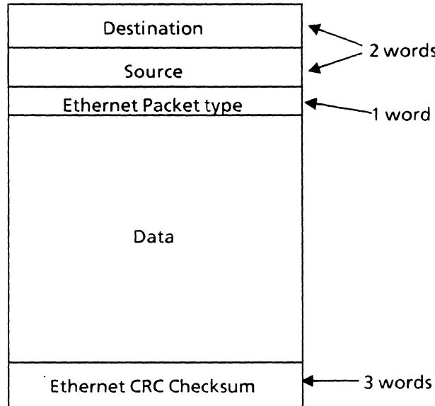
Figure 2.5 Ethernet packet
