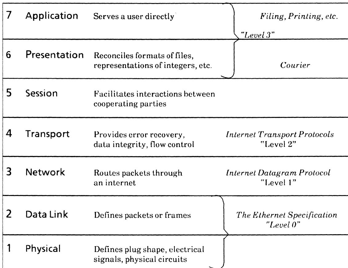
Figure 2.3 Open Systems Interconnect Reference Model
