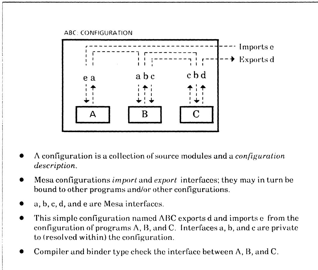
Figure 3.3 Mesa configurations hiding interfaces
