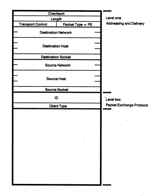
Figure 8.1 The packet exchange protocol packet
