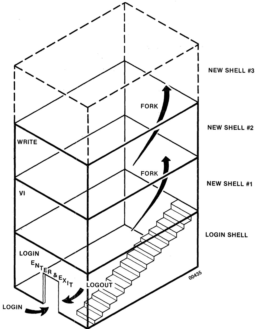
Figure 5-1 Representation of the Fork Process
