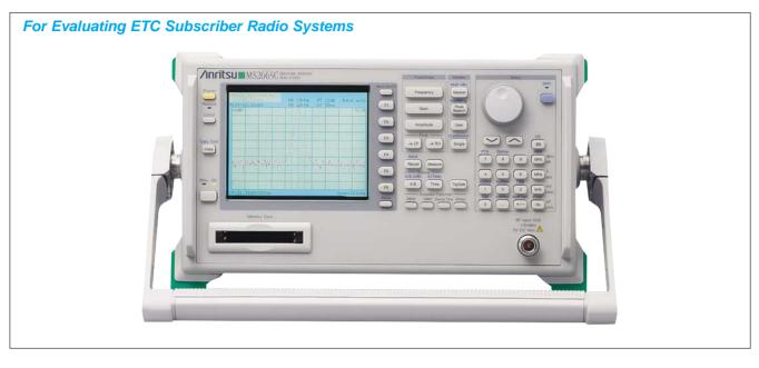
The MS2665C is a compact, lightweight, and low-price spectrum analyzer that covers a frequency range of 9 kHz to 21.2 GHz. It has superior basic performance such as a high C/N ratio, low distortion, and high frequency/level accuracies and is easy to operate. A large selection of options is provided to handle a wide range of applications at a reasonable cost.
