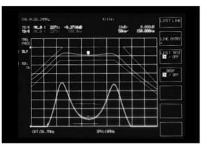
Filter pass/fail evaluation using limit test
