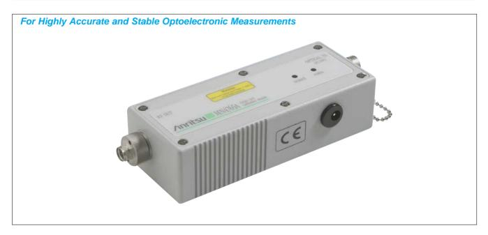
The MN4765A is a characterized, unamplified photodiode module. It is used as an optical receiver with the 37000D series VNAs to perform highly accurate and stable optoelectronic measurements of both modulators (E/O) and photoreceivers (O/E) to 65 GHz.
