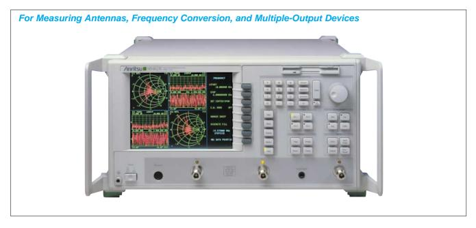
The MS462XC series of RF vector network analyzers are configured as direct-access receivers for antenna, frequency conversion, and multiple output device measurements. The MS462XC offers ultimate flexibility to meet most receiver measurement needs while maintaining the ability to measure all four S-parameters with the addition of a reflectometer setup at the front end of the receiver.
