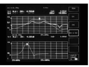
Spurious measurement using alternate sweeping
