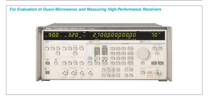
The MG3633A has excellent frequency resolution, frequency switching speed, signal purity, and a high output level, in addition to amplitude, frequency, and phase modulation functions. Also, sweep functions are provided for carrier frequency, output level, and modulation frequency so an appropriate sweep can be performed for various devices to be measured.
