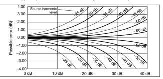
This chart assumes full reflections of a single source harmonic at the DUT input. Multiple harmonics can cause additional measurement uncertainty.
