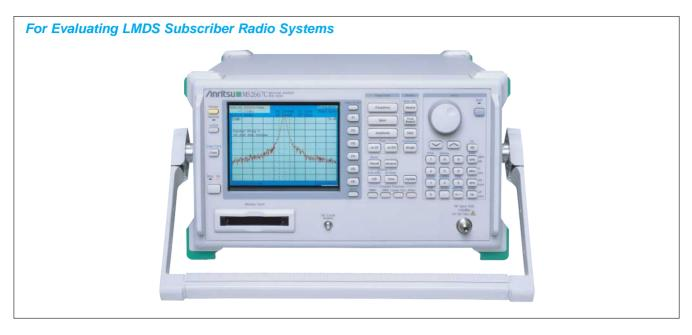
The MS2667C is a compact, lightweight, and low-price spectrum analyzer that covers a frequency range of 9 kHz to 30 GHz. It has superior basic performance, such as a high C/N ratio, low distortion, and high frequency/level accuracies, and is easy to operate. A large selection of options is provided to handle a wide range of applications at reasonable cost.
