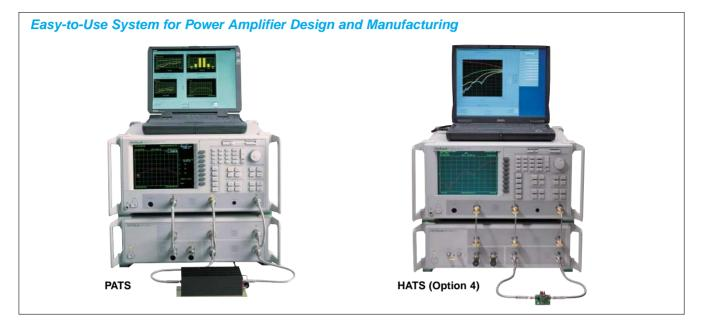
The ME7840A Power Amplifier Test System (PATS) is a flexible, easy-to-use system for base station power amplifier testing and with the introduction of the new option 4 Handset Amplifier Test Set (HATS) it now provides full coverage to handle all of your power amplifier testing needs.
