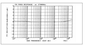
**Figure 5. FM Modulation Frequency Characteristics**
