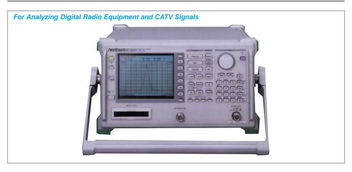
The MS2661C Portable Spectrum Analyzer is for signal analysis of radio and other equipment related to improving frequency usage efficiency, higher modulation, and digitalization. The MS2661C is a synthesized spectrum analyzer covering a wide frequency range from 9 kHz to 3 GHz and it has superior basic performance such as high C/N ratio, low distortion, and a high frequency/level accuracies.
