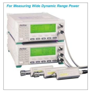
The ML2430A series Power Meters combine the advantages of thermal meter accuracy, diode meter speed, and peak power meter display graphics. The result is a single instrument that achieves 90 dB dynamic range with a single sensor. The ML2430A series includes graphics display capability as a standard feature. The ruggedized housing and optional high-capacity NiMH battery bring convenience and accuracy to field service applications.
