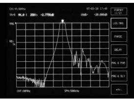
Filter out-of-band attenuation measurement
