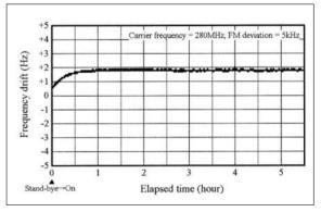
Carrier wave frequency stability at frequency modulation
