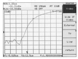
High-speed time domain measurement (TS = 12.5  $\mu$ s)
