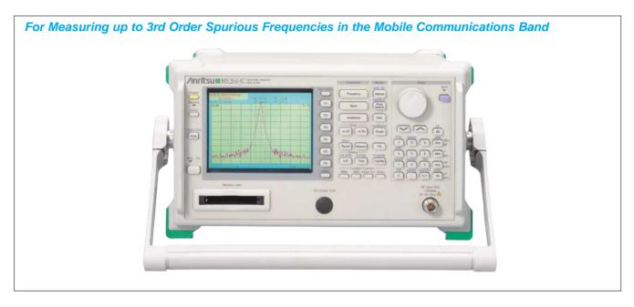
The MS2663C covers a frequency range of 9 kHz to 8.1 GHz. This allows measurement of spurious frequencies of up to three times greater than the frequency bands used worldwide for mobile communications. The MS2663C has superior basic performance such as high C/N ratio, low distortion, and high frequency/level accuracies and is easy to operate.
