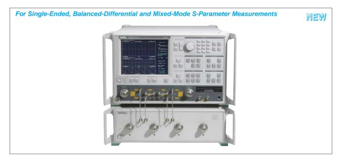
The Microwave Multi-Port Balanced VNA consists of a 37000D Lightning VNA, a multi-port test set, and the Navigator<sup>™</sup> Multi-Port software (external PC is required and is not included). The multi-port test set is a 2x4 switch matrix that allows either port on the VNA to connect with any of the 4 ports on the test set. The easy-to-use Navigator<sup>™</sup> Multi-Port software provides full step-by-step direction, simplifying calibration, and speeding measurement throughput.
