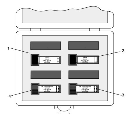
Figure 11-2. Model 3751R GPC-7 Calibration Kit
