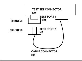
Figure 7-3. Use of PEAs to Establish Test Ports
