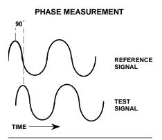
**Figure 3-6.** Signals with a 90 Degree Phase Difference
