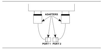
**Figure 7-2.** Using Adapters on the Test Ports
