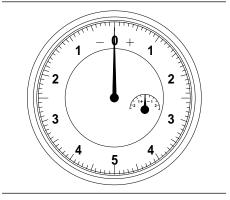
Figure 11-5. Pin Depth Gauge
