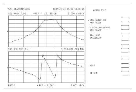
Figure 6-2. Single Channel Display, Log Magnitude and Phase
