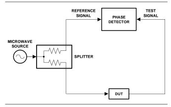
Figure 3-4. Splitting the Microwave Signal
