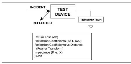
Figure 3-2. Reflection Measurements
