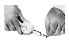
**Step 4.** While holding the gauge as shown, press the Ref Flat firmly against the end of the exposed center pin.
