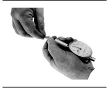
**Step 18.** Install the female adapter over the center pin and screw it into the locking ring, and tighten the outer ring until it is snug against the housing.
