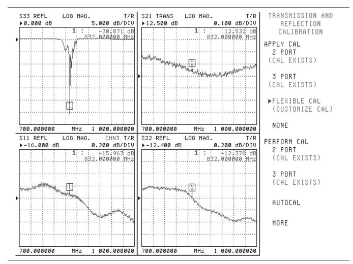
Figure 7-9. Example Comparing Flexible Calibration Results with Full 3-Port Calibration Results
