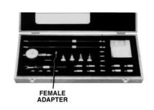
**Step 17.** Remove the 01-223 Female Adapter ("F ADAPTER FOR PIN GAUGE") from the kit.
