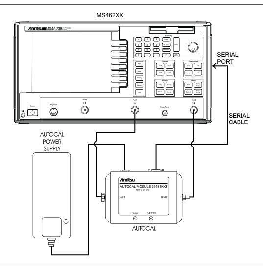
Figure 9-2. AutoCal Equipment Setup
