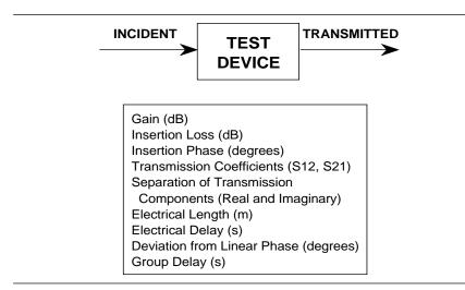
Figure 3-1. Transmission Measurements
