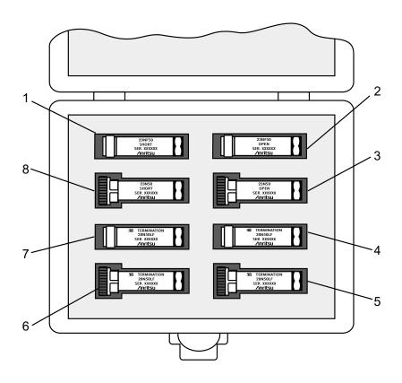
Figure 11-3. Model 3753R Type N Calibration Kit
