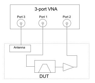
Figure 7-8. 3-Port VNA Measuring a 3-Port Device
