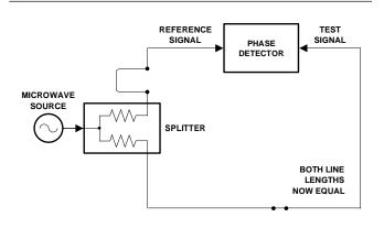
Figure 3-11. Split Signal where Paths are of Equal Length
