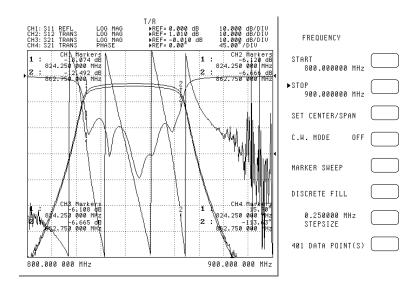
Figure 6-6. Four Channel Trace Overlay
