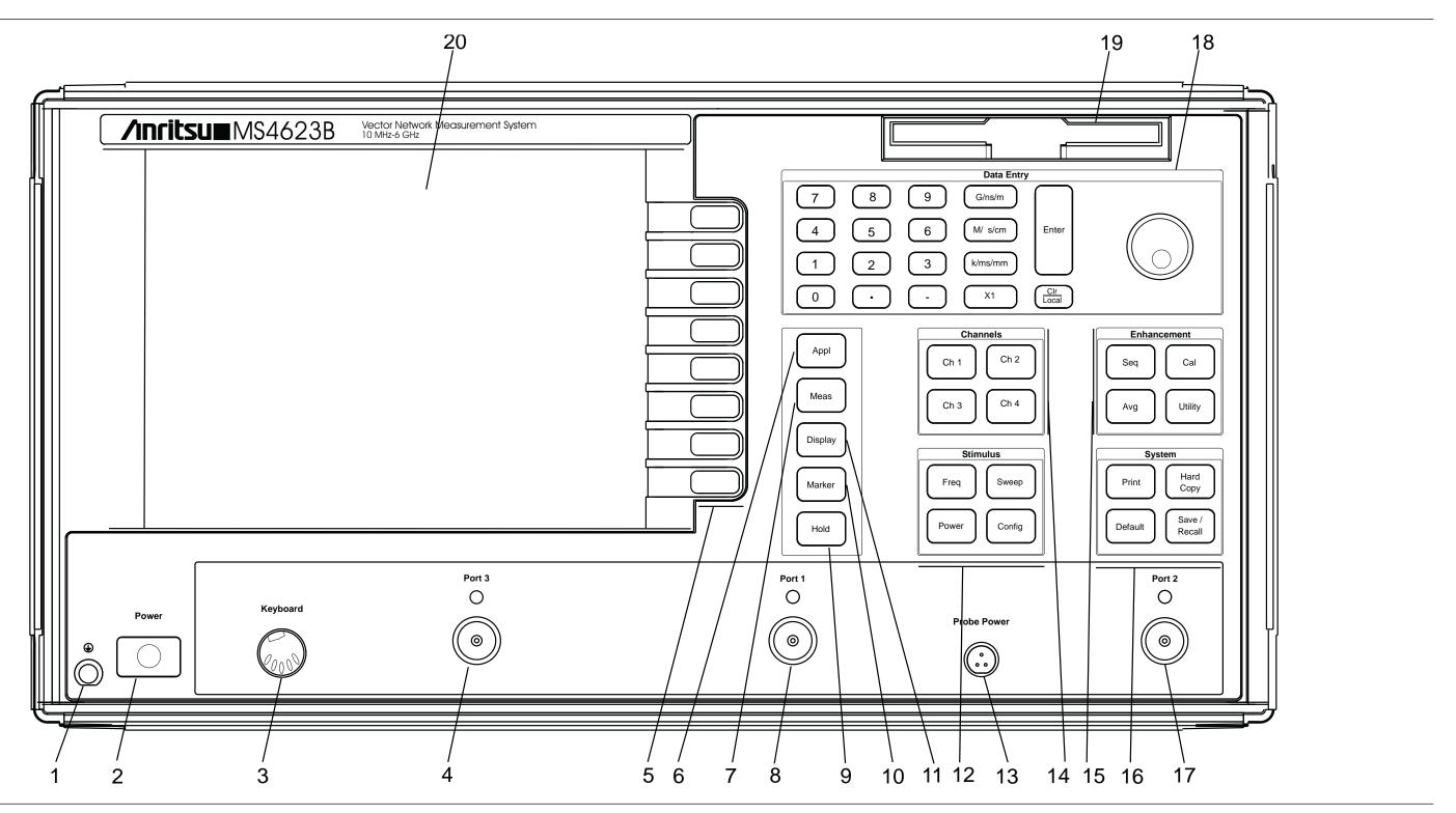
Figure 4-1. MS4623B Network Analyzer Front Panel Controls and Connector
