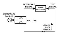
**Figure 3-7.** Split Signal where a Length of Line Replaces the DUT
