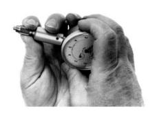
**Step 2.** Push the outer locking ring towards the gauge to expose the center pin.
