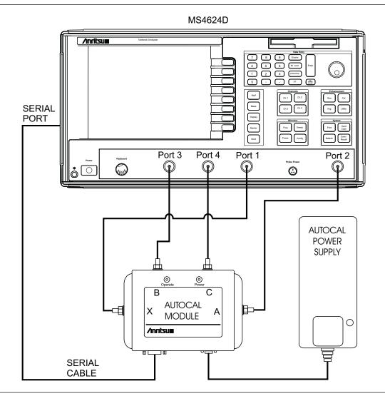
Figure 9-3. 4-Port AutoCal Equipment Setup
