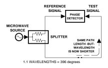
**Figure 3-9.** Split Signal where Path Length is Longer than One Wavelength
