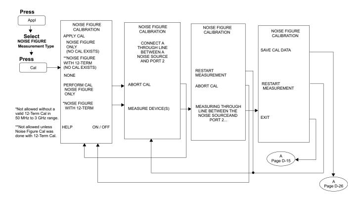
Figure D-18. Calibration Key Menu Map (Noise Figure)(1 of 1)
