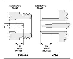
Figure 11-4. N Connector Pin Depth
