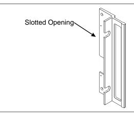
Figure 2-1. Rack Mount Handle Showing Slotted Opening
