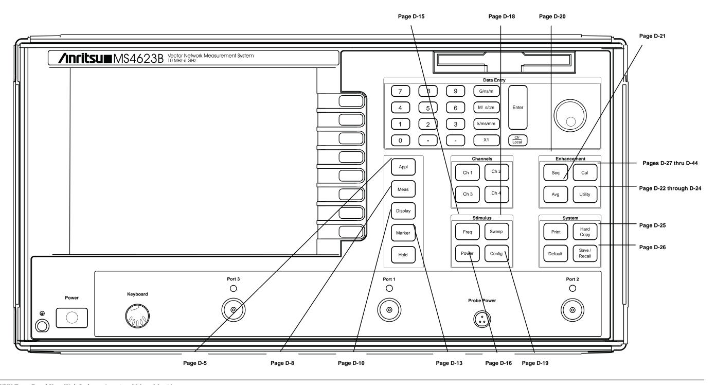
Figure D-1. MS462XXX Front Panel Keys With Index to Associated Menu Map(s)
