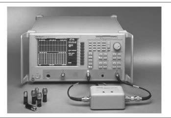
Figure 7-2. Two-Port AutoCal System Setup
