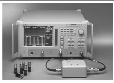
Figure 3-1. MS462XX with Two-Port AutoCal Module
