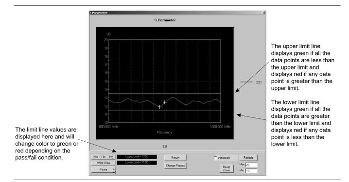
Limit lines are displayed on the S-parameter test screen as shown below.
