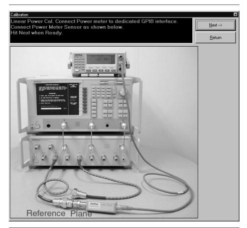
**Step 2.** Before the calibration begins, you will be prompted to zero and calibrate the power meter. Refer to the procedures outlined in your power meter's documentation to ensure that the power meter is properly calibrated and that any offset feature is turned off.
