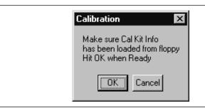
**Step 17.** Connect the broadband Load to Test Port 1 on the test set and click OK.
