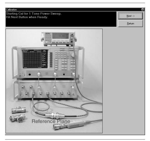
*Step 23.* Connect a throughline between Test Port 1 and Test Port 2 on the test set.
