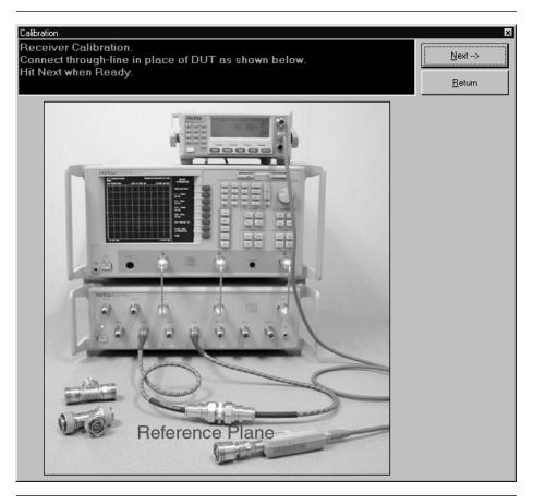
*Step 6.* Press Next to perform the Receiver Calibration.
