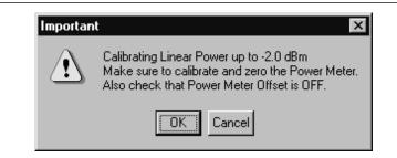
*Step 3.* Reconnect the power sensor to the power reference plane and click OK.
