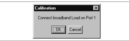
*Step 18.* Connect the Open to Test Port 1 on the test set and click OK.
