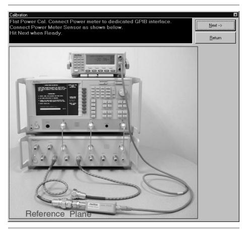
The Flat Power calibration takes less than one minute to complete. It calibrates the output power at the reference plane for both of the Scorpion's internal sources (power out of Port 1, then Port 3) according to the target power across the frequency range set in the calibration specification file. When the test completes, the Next button will become available.
