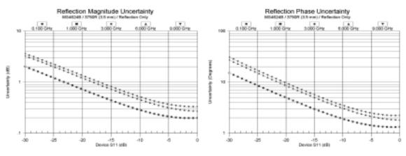
Reflection Measurements: 3.5 mm Connectors
