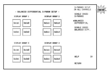
**Liquid Crystal Display:** A Color 8.4" Thin Film Transistor (TFT) LCD display is standard on all units. The default color configuration is as follows: graticules are displayed in green, measurement data in red, background in black, markers and limits in blue, and overlaid trace data in yellow. Trace data stored in memory are displayed in green.
