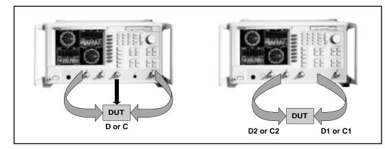
Measurement of 3 and 4-port single ended S-parameters are required in order to perform the mixed-mode conversion, which generates results as if the ports were being driven in pairs.
