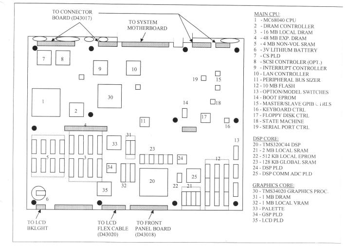
FIGURE 1 - CPU Board Block Diagram
