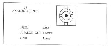
FIGURE 9 – Analog Output Connector Diagram
