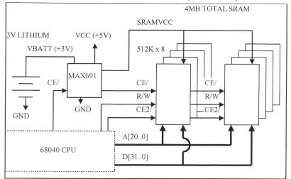
FIGURE 16 - Battery Backed SRAM
