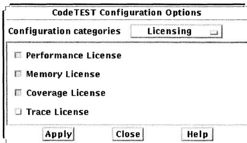
To load and view saved data that was acquired with any or all of the CodeTEST tools, you need only one license of any type. If you load a data file without first selecting a license, CodeTEST will automatically determine what licenses are available and select one for you.
