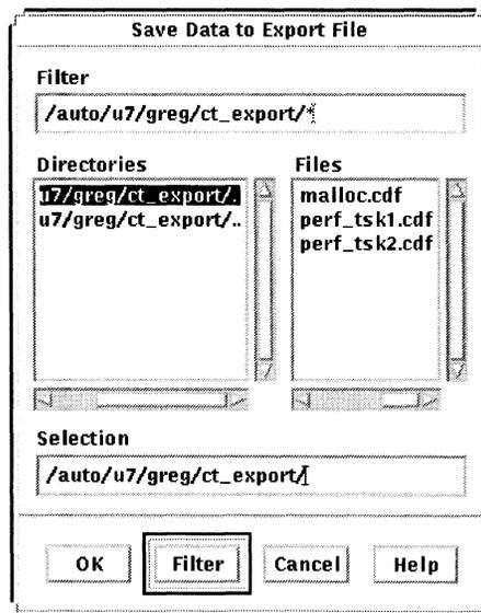
You can import CodeTEST CDF files into most popular spreadsheet programs for post-processing measurement data, or into publishing programs for producing printed reports.
