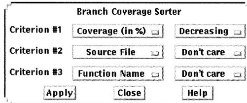
With the % Coverage column sorted in decreasing order, functions with the highest levels of coverage are arranged at the top of the table.
