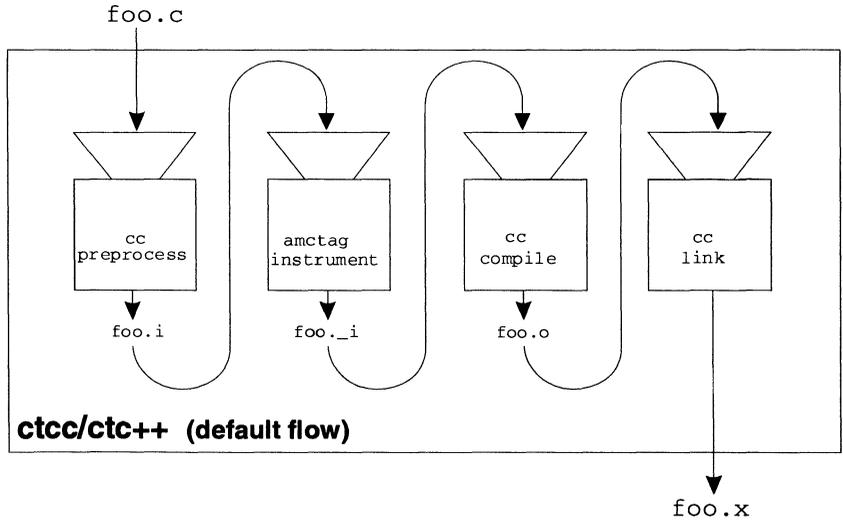
By default, `ctcc/ctc++` first invokes your compiler's driver to perform C/C++ preprocessing, then calls the instrumenter (`amctag`) to insert CodeTEST tags into your preprocessed code, and then sends the instrumented code back to your compiler's driver to complete the build.
