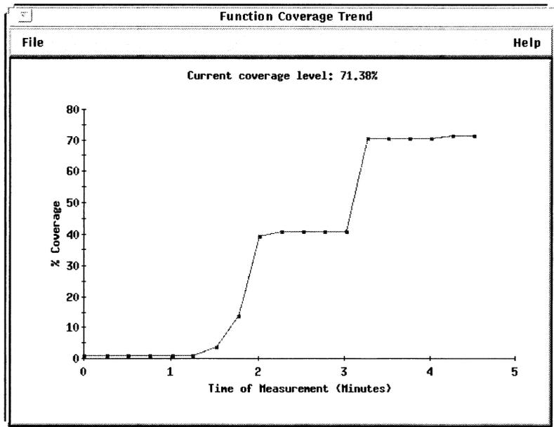
With the Coverage Trend view, you can easily identify *dead spots* in your testing, where no new coverage is being achieved. By modifying your test stimulus accordingly, you may be able to reduce your testing time substantially, while still testing just as thoroughly.
