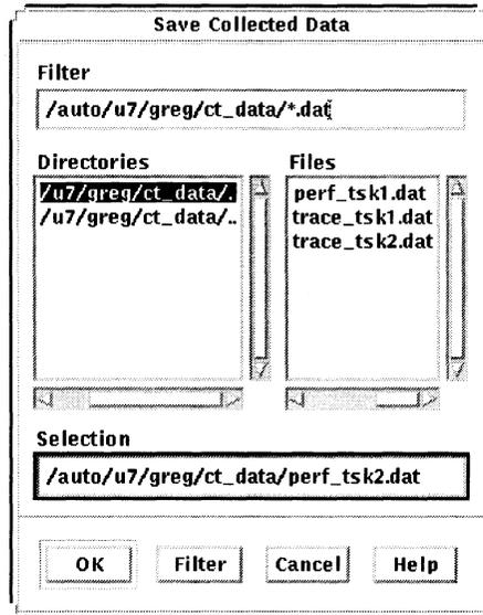
To save a file, first select a directory in the Directories scroll box. This places the directory path in the Filter box. If you wish, you can specify a file filter in the Filter box (using the \* and ? wildcard characters). Click the Filter button to put your filter into effect. In the example above, the filter /auto/u7/greg/ct\_data/\*.dat was applied.
