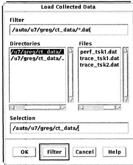
To load a file, first select the directory in the Directories scroll box. This places the directory path the Filter box. If you wish, you can also specify a file filter in the Filter box (using the \* and ? wildcard characters). Click the Filter button to put your filter into effect. In the example above, the filter /auto/u7/greg/ct\_data/\*.dat was applied.
