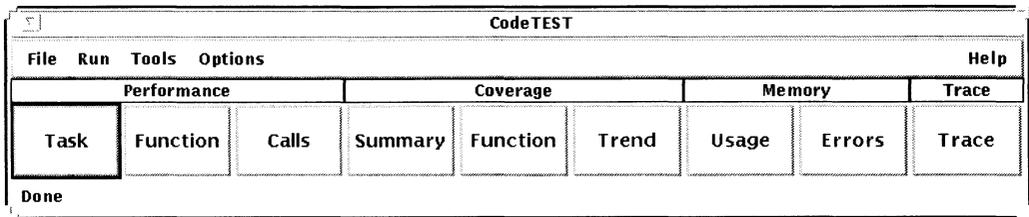
The status line at the bottom of the toolbar displays self-explanatory operational and error messages. To see a listing of any error messages generated during your session, select **Error Log** from the **Tools** menu. Appendix B provides troubleshooting information for the CodeTEST error messages.
