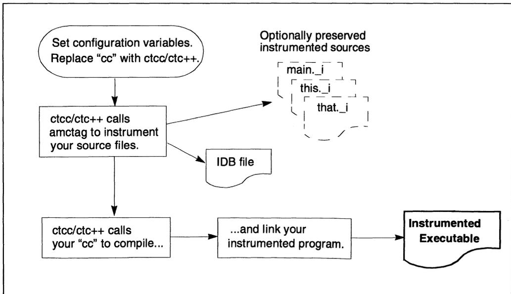
By defining a set of variables to adapt the instrumenter to your environment, and substituting `ctcc` or `ctc++` wherever “`cc`” appears in your makefile or build script, you can automatically instrument your sources with each compilation, link in the necessary CodeTEST libraries, and assign memory locations to the two CodeTEST port addresses. This approach is designed to ease instrumentation into your environment with minimal change to existing procedures.
