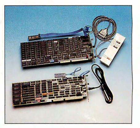
Hardware-assisted debuggers like AT Probe (top) and Periscope III (bottom) can significantly reduce debugging time—for a price.
