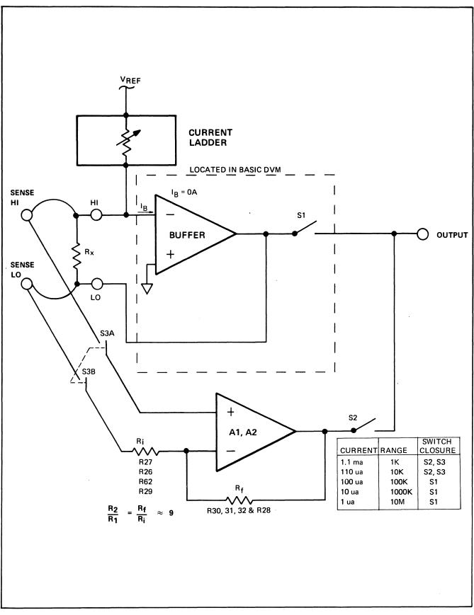
FIGURE 15. BLOCK DIAGRAM OF OHM CONVERTER
