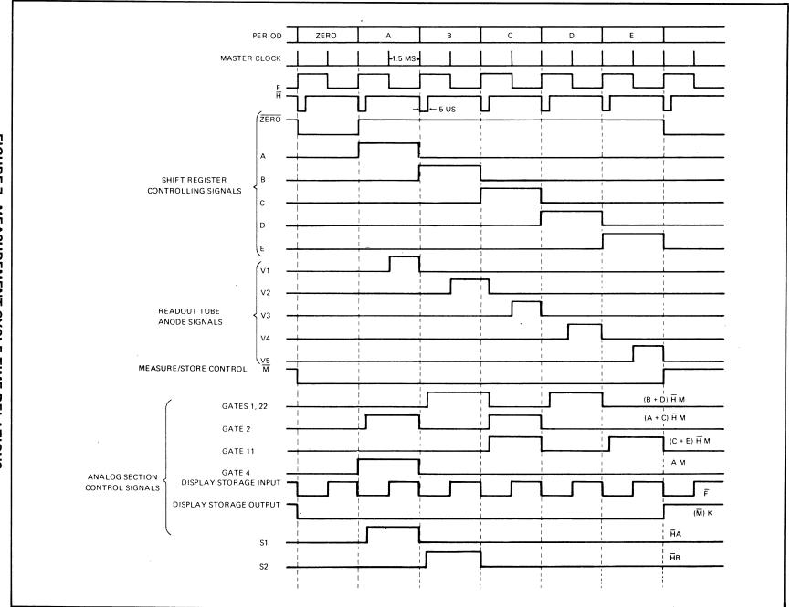
FIGURE 7. MEASUREMENT CYCLE TIME RELATIONS
