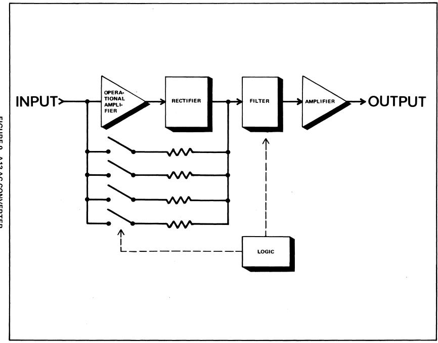
FIGURE 9. A13 AC CONVERTER
