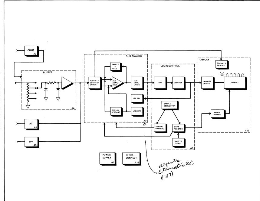
Figure 10. BLOCK DIAGRAM
