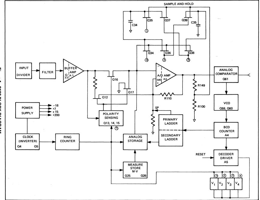
Figure 1. 8100 BLOCK DIAGRAM
