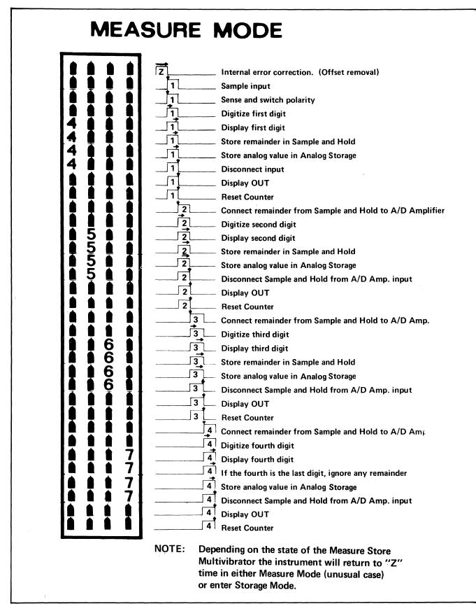
Figure 5. 8100 DISPLAY SEQUENCE, MEASURE MODE
