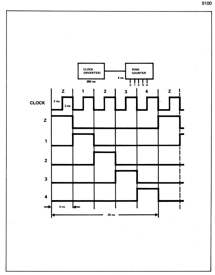
Figure 4. 8100 TIMING DIAGRAM
