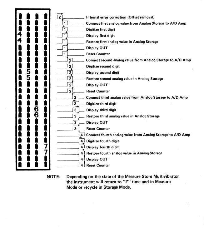
Figure 7. 8100 DISPLAY SEQUENCE, STORAGE MODE
