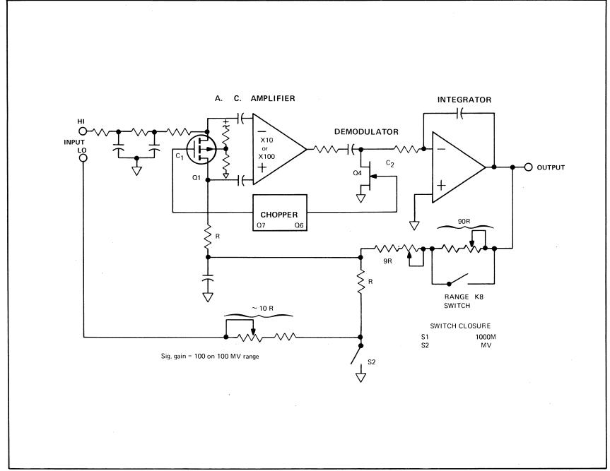
FIGURE 14. BLOCK DIAGRAM OF MILLIVOLT CONVERTER
