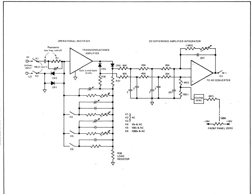
FIGURE 13. BLOCK DIAGRAM AC CONVERTER
