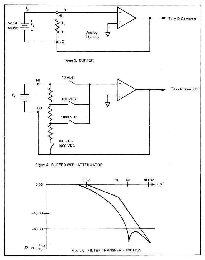
that establish a unity gain frequency of 3 Hz. This roll off of the gain of the buffer provides high frequency filtering by attenuating the AC signals inside the buffer and presenting a reduced version of the AC signal input to the A-D Converter. The frequency characteristics are shown in Figure 5. A notch filter is provided at 60 Hz and three pole response is present above 30 Hz. As the figure shows, for all frequencies above 50 Hz, the rejection of AC signal at the input is greater than 60 db.
