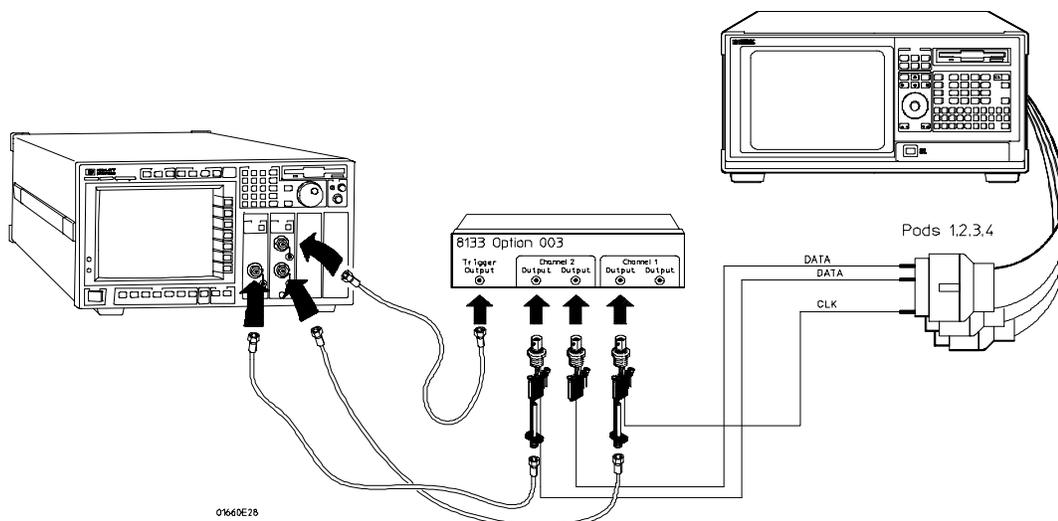
3 Activate the data channels that are connected according to one of the previous tables.
