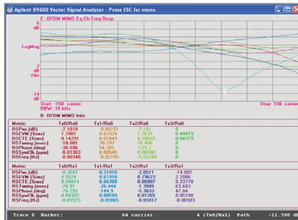
**Figure 26. Trace D displays the equalizer frequency response for all detected ports of a 4x2 MIMO system. The marker readout indicates problems with the Tx0/Rx1 path. The MIMO info table shows that this path has high RS EVM. Note the matching color-coding between the two traces.**
