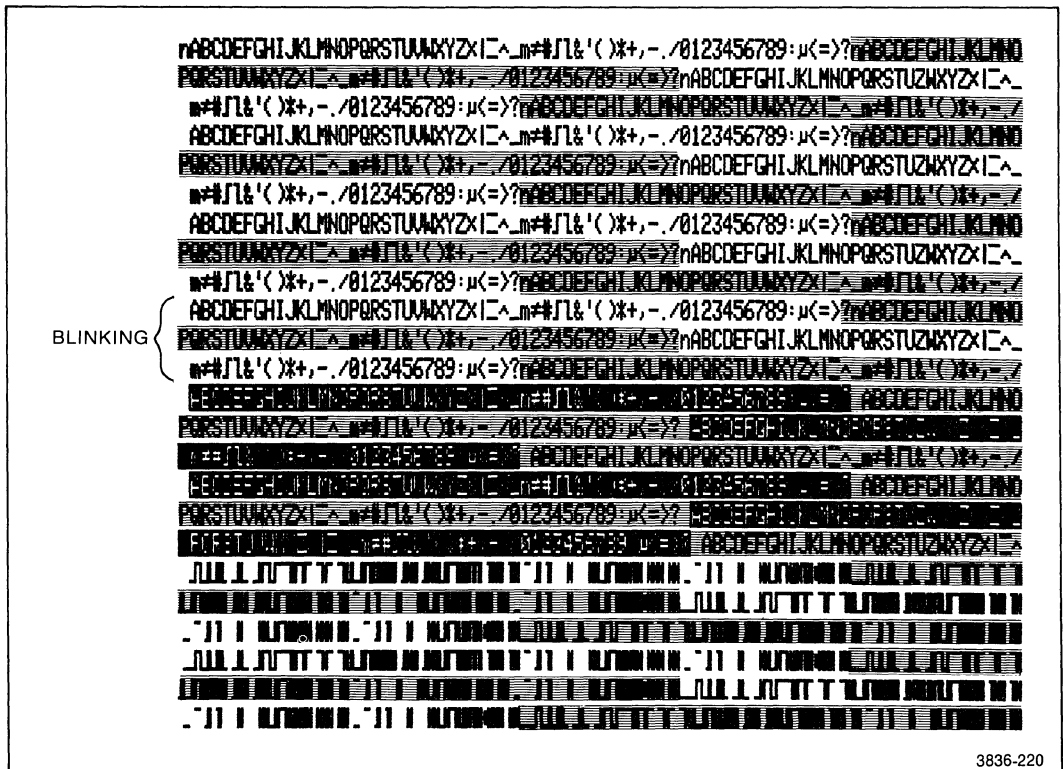
Figure 8-2. All-character diagnostic display.
