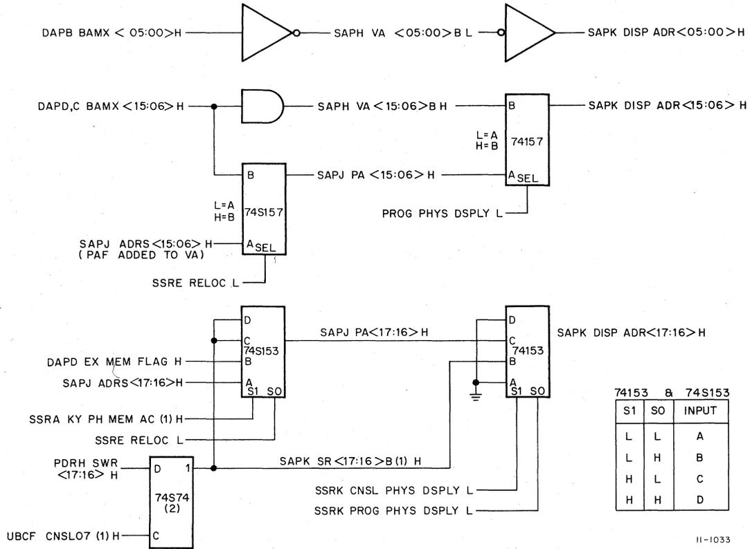
Figure 3-3 Sources of ADDRESS Display, Simplified Diagram
