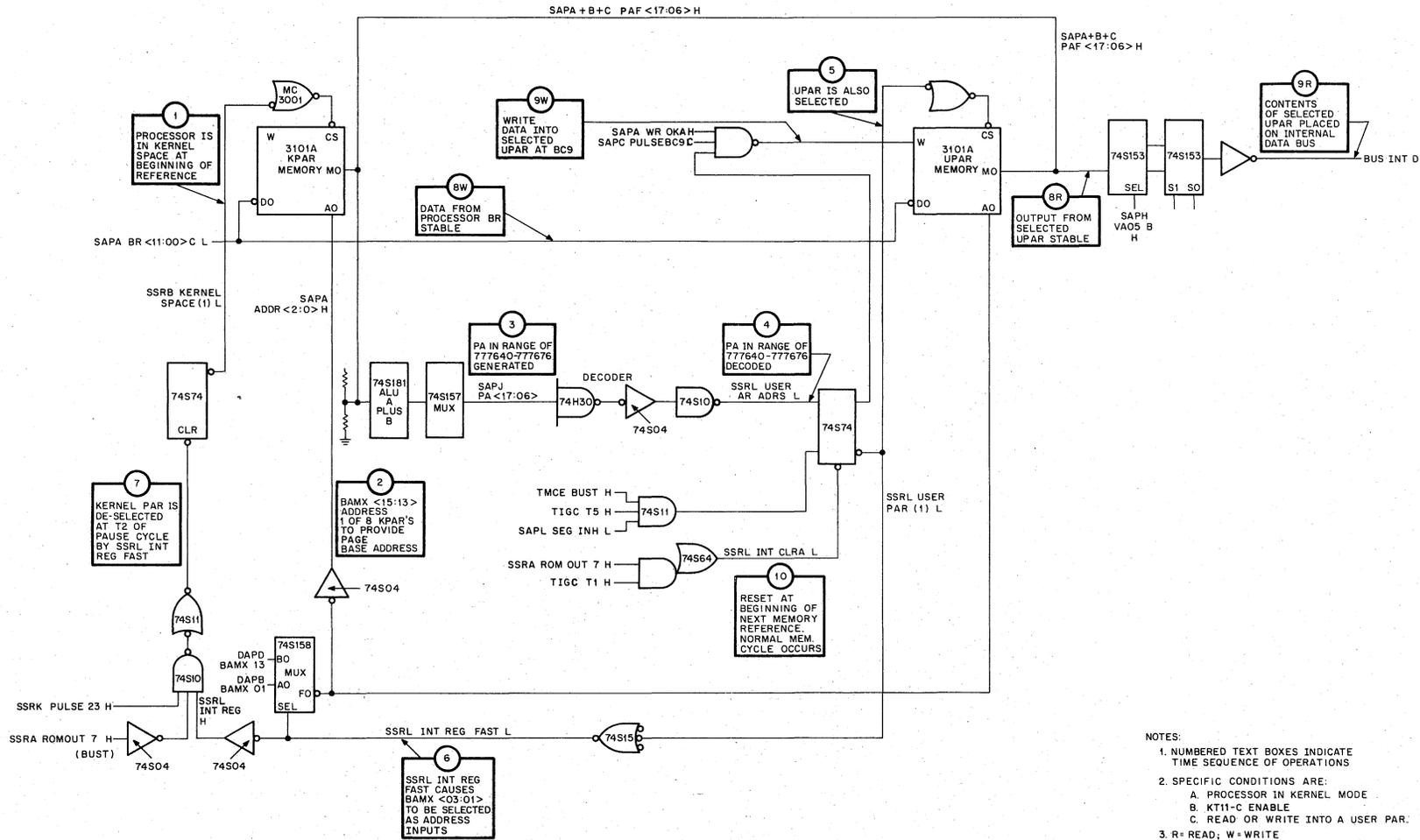
Figure 3-9 Internal Register Access Sequence, Simplified Diagram
