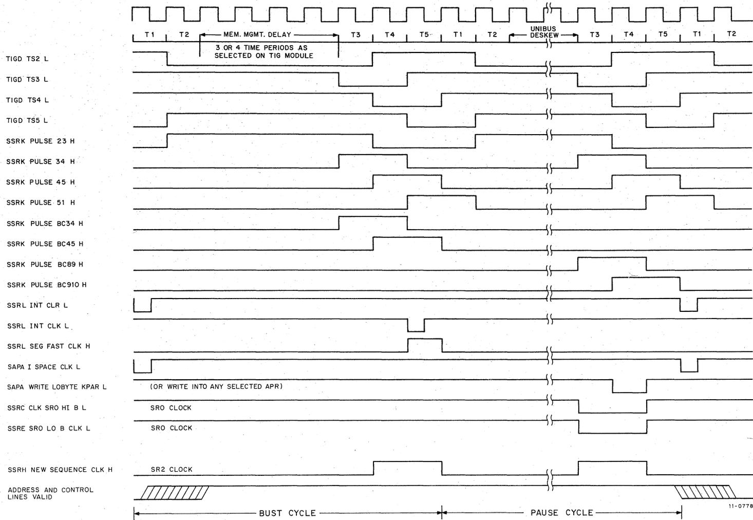
Figure 3-7 KT11-C Timing Diagram
