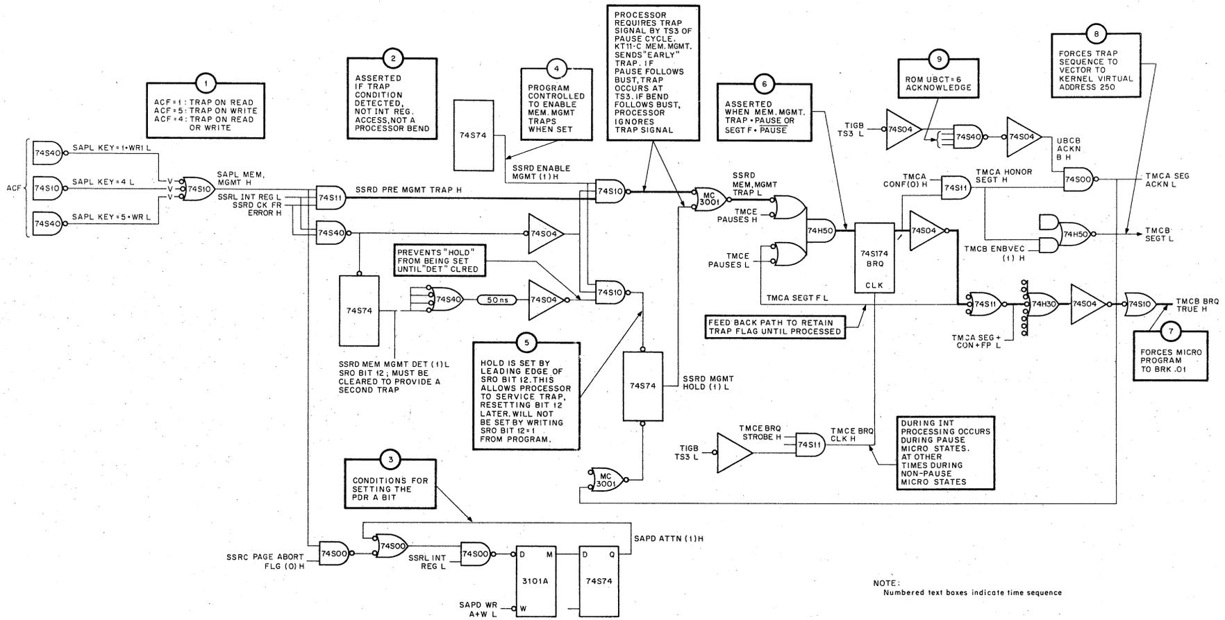
Figure 3-5 KT11-C/KB11-A Trap Control Sequence
