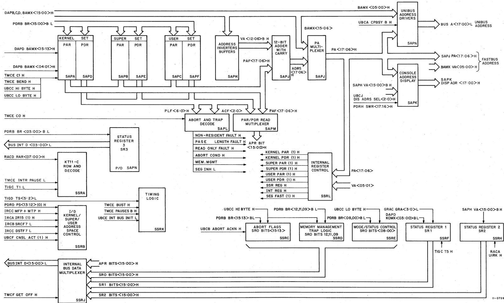
Figure 3-2 KT11-C Memory Management Unit, Block Diagram
