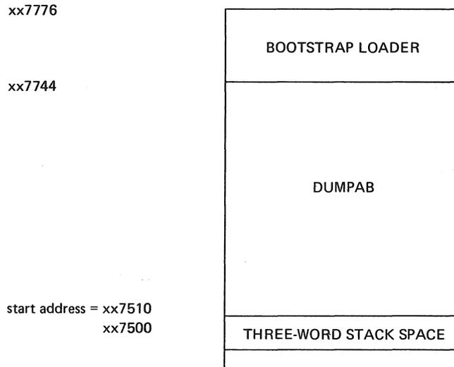
The DUMPAB program (for systems without a switch register) is 82(10) words long. When used in absolute format the storage map is:
