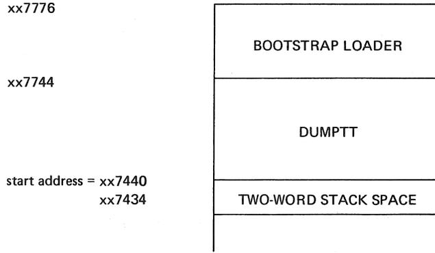
The DUMPAB program (for systems with a switch register) is 65(10) words long. When used in absolute format the storage map is:
