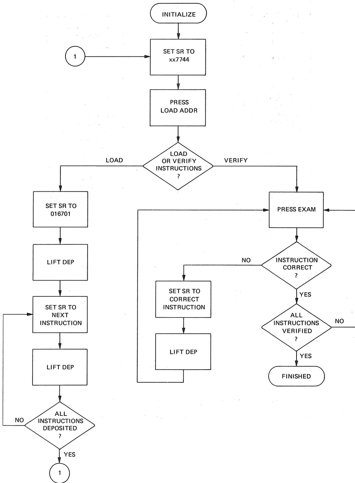
Figure 6-2 Loading and Verifying the Bootstrap Loader
