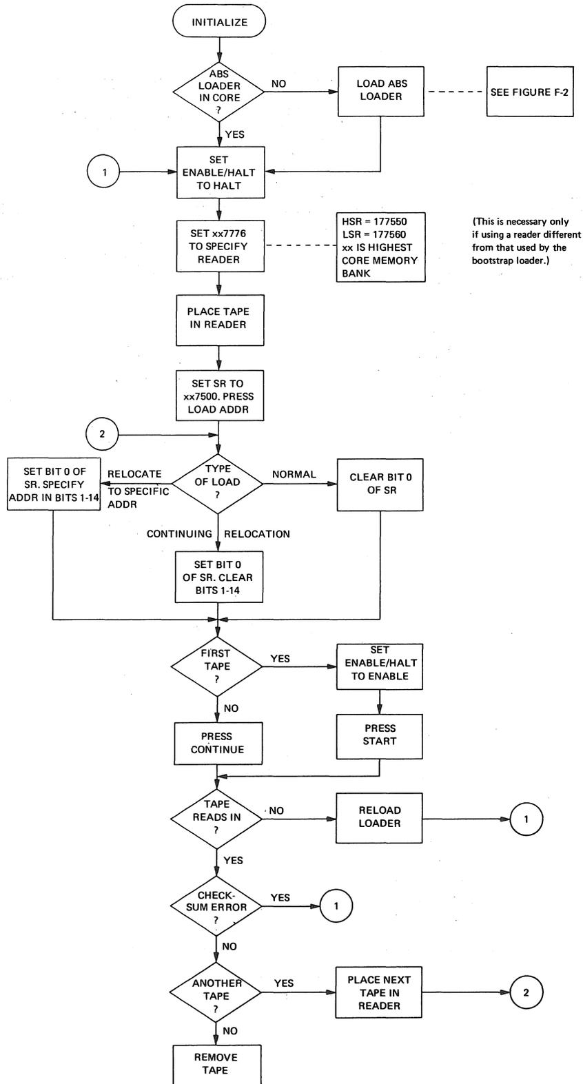
Figure F-3 Loading with the Absolute Loader
