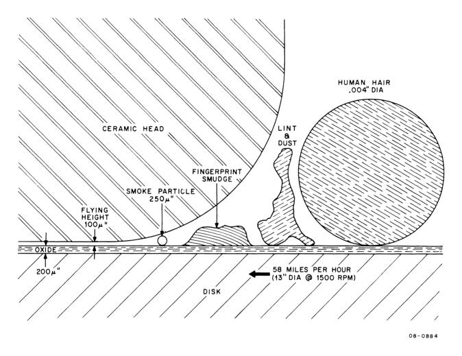
Figure 1-8 Relationship of Disk Head, Disk, and Contaminants
