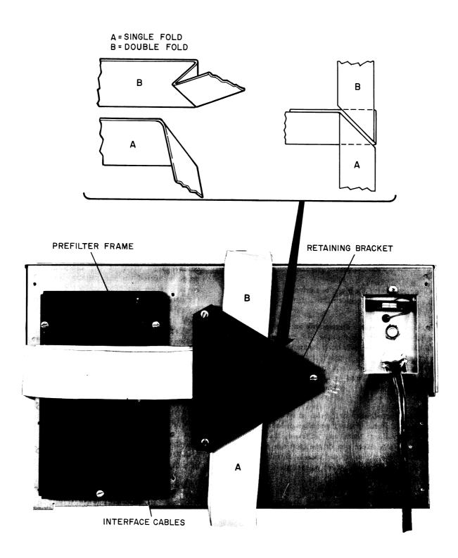
Figure 2-4 RK8/E Interface Cable Installation
