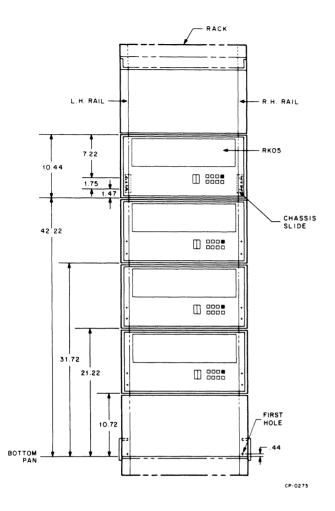
Figure 2-3 Chassis Slide Mounting
